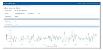
Both frequency and time domain spectral captures can be graphically displayed within the web interface, with controls for scale and range-zoom via simple click and drag. As with other data, the sweep and time data can be filtered by Node ID, campaign, date/time, antenna input and spectral processing, and also output to CSV.
