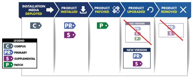
FIGURE 3 - The Lifecycle of software on an endpoint documented by SWID tags. Souce: NISTIR 8060
