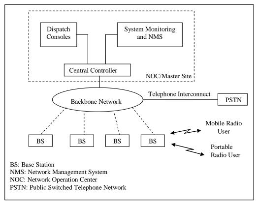
Figure 2-1. Typical Configuration of a Trunked Radio System
