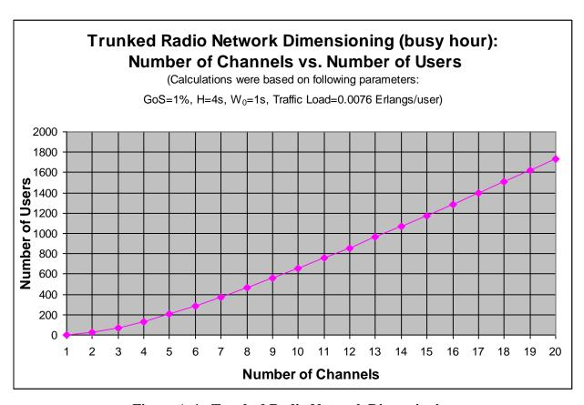
Figure A-1. Trunked Radio Network Dimensioning
