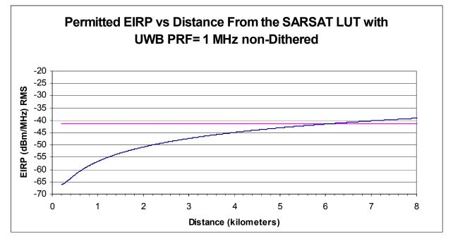
Figure 4-15a. Maximum Permitted UWB EIRP for non-Dithered PRF of 1MHz (UWB Height =30m).
