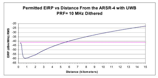
Figure 3-5. Maximum EIRP vs. Distance for 2 Meter UWB Antenna Height.
