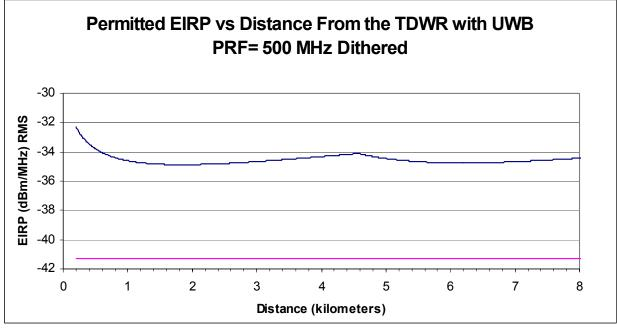
Figure 4-23 Maximum Permitted UWB EIRP for Dithered PRF (UWB Height = 2m).
