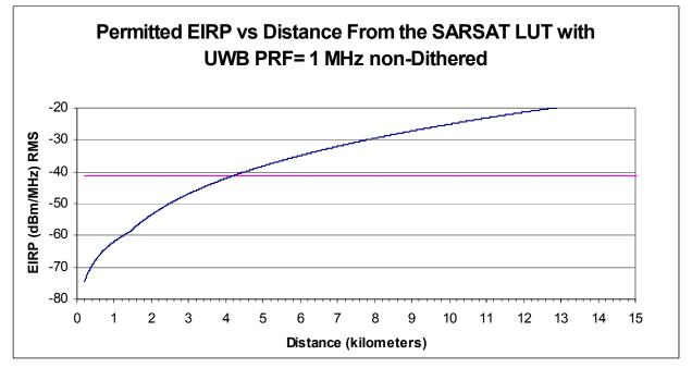
Figure 4-13b. Maximum Permitted UWB EIRP for non-Dithered PRF of 1 MHz (UWB Height = 2m).
