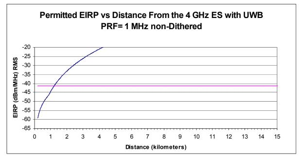
Figure 44-18d. Maximum Permitted UWB EIRP for non-Dithered PRF of 1 MHz (UWB Height = 2 m).
