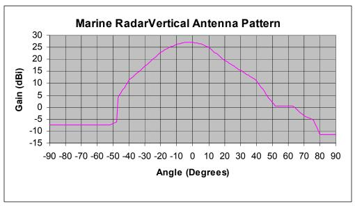
Figure A-14. Marine Radar Vertical Antenna Pattern.
