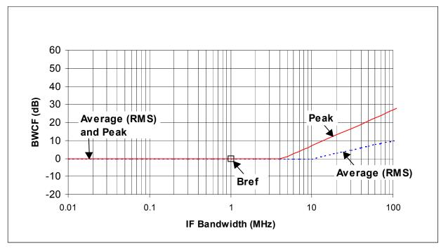
Figure 3-2. BWCF for 10 MHz PRF Non-dithered UWB Signal.
