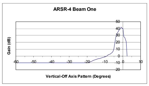
Figure A-4. ARSR-4 Beam One Vertical Antenna Pattern.
