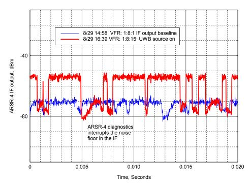
Figure C-3. ARSR-4 IF Output for Baseline Noise Level (UWB Signal off) and UWB Signal on for Site #2 (2.1 km). Peak Detected in 1 MHz Resolution and Video Bandwidth.
