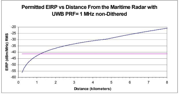
Figure 4-25 Maximum Permitted UWB EIRP for non-Dithered PRF of 1 MHz (UWB Height = 2m).
