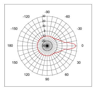
Figure B-13. Parabolic, SARSAT LUT Antenna Pattern.
