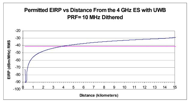
Figure 4-20a. Maximum Permitted UWB EIRP for Dithered PRF of 10 MHz (UWB Height = 30m).
