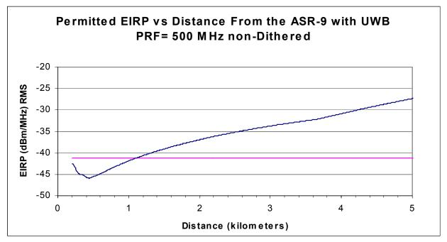
Figure 4-10. Maximum Permitted UWB EIRP for non-Dithered PRF of 500MHz (UWB Height = 2m).
