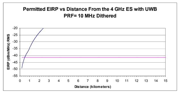
Figure 4-19d. Maximum Permitted UWB EIRP for Dithered 10 MHz UWB (Height = 2m).
