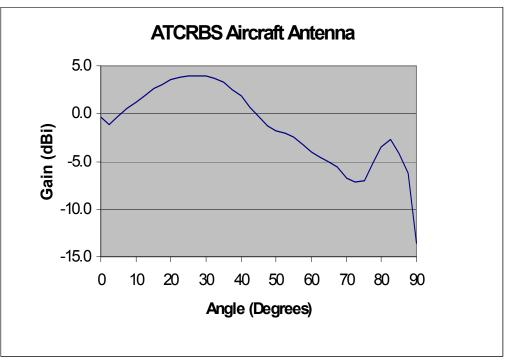
Figure A-9. ATCRBS Transponder Vertical Antenna Pattern.
