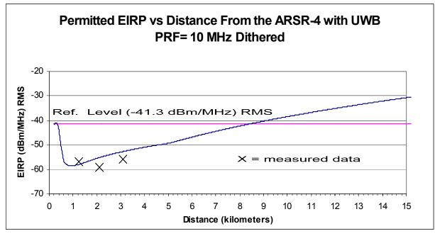
Figure 3-7. Comparison of Measured and Predicted Maximum Permitted EIRP versus Distance From ARSR-4 for 10 MHz Dithered UWB Signal
