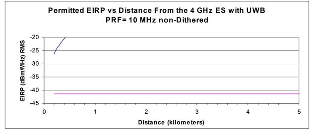
Figure 4-18c. Maximum Permitted UWB EIRP for non-Dithered PRF 10 MHz (UWB Ht = 2m).
