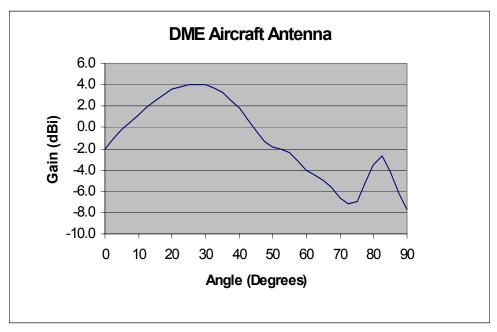
Figure A-11. DME Interrogator Vertical Antenna Pattern.
