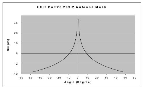
Figure A-12. Earth Station Antenna Pattern.
