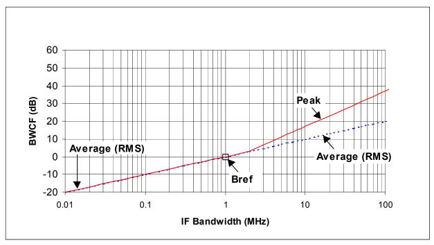
Figure 3-4. BWCF for 10 MHz Dithered UWB Signal.
