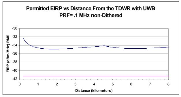
Figure 4-21. Maximum Permitted UWB EIRP for non-Dithered PRF of 1 MHz (UWB Height = 2m).
