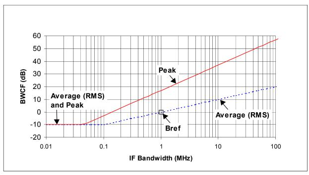
Figure 3-1. BWCF for 0.1 MHz PRF Non-dithered UWB Signal.
