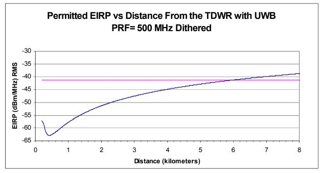
Figure 4-24 Maximum Permitted UWB EIRP for UWB Height =30 m.
