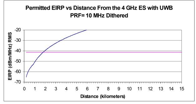
Figure 4-19a. Maximum Permitted UWB EIRP for Dithered PRF of 10 MHz (UWB Height = 2m).
