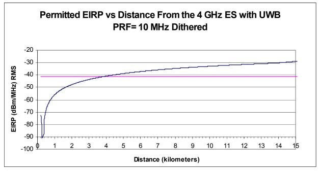
Figure 4-20b. Maximum Permitted UWB EIRP for Dithered PRF of 10 MHz (UWB Height = 30m).
