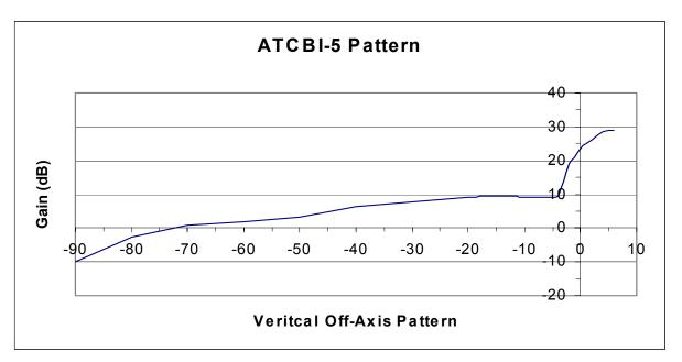
Figure A-8. ATCRBS Interrogator Vertical Antenna Pattern Used in Conjunction with ARSR-4.
