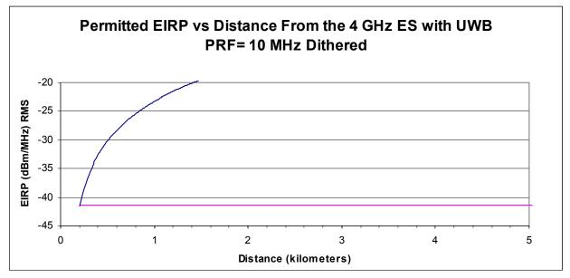
Figure 4-19c. Maximum Permitted UWB EIRP for Dithered PRF of 10 MHz UWB Height = 30m.
