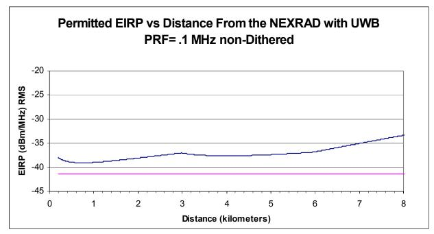
Figure 4-1. Maximum Permitted UWB EIRP for non-Dithered PRF of 0.1 MHz (UWB Height = 2m).
