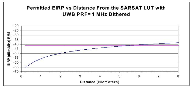
Figure 4-16a. Maximum Permitted UWB EIRP for Dithered PRF of 1MHz (UWB Height =30m).
