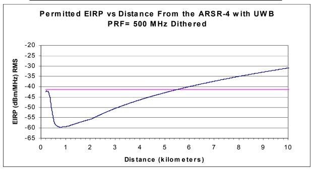
Figure 4-7. Maximum Permitted UWB EIRP for Dithered PRF (UWB Height = 2m).
