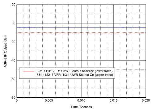
Figure C-6. ASR-8 IF Output for Baseline Noise Level (UWB Signal Off) and UWB Signal on for Site #1 (0.4 km). Peak Detected with 1 MHz Resolution Bandwidth and 10 Hz Video Bandwidth, RMS Noise Level.
