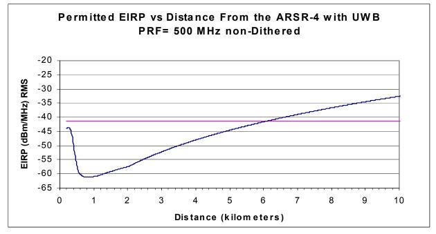
Figure 4-6. Maximum Permitted UWB EIRP for non-Dithered PRF of 500MHz (UWB Height = 2m).
