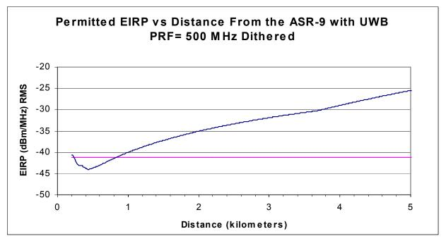
Figure 4-11. Maximum Permitted UWB EIRP for Dithered PRF (UWB Height = 2m).
