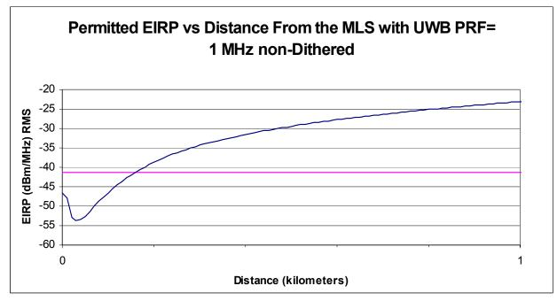
Figure 4-13. Maximum Permissible UWB EIRP for non-Dithered 1 MHz PRF (UWB Height = 2 m).
