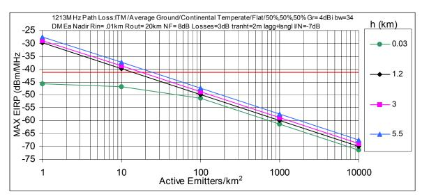
Figure 5.5.5 DME (Airborne Interrogator)
