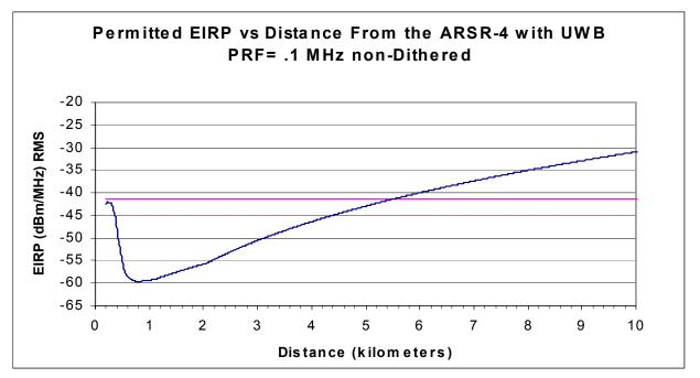
Figure 4-5. Maximum Permitted UWB EIRP for non-Dithered PRF of 0.1 MHz (UWB Height = 2m).
