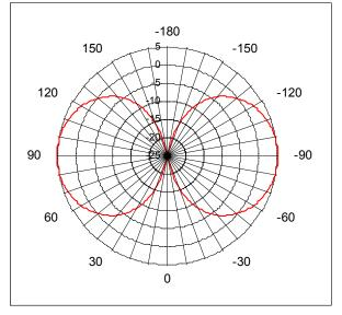
Figure B-15. Dipole Array Antenna Pattern.
