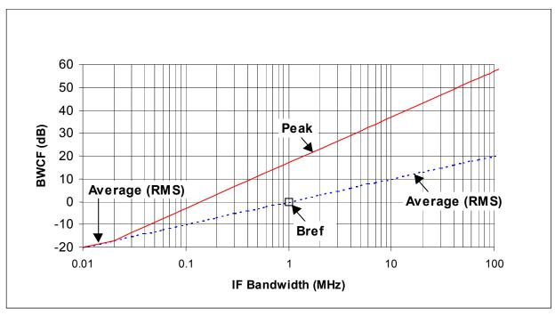
Figure 3-3. BWCF for 0.1 MHz PRF Dithered UWB Signal.
