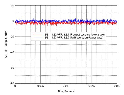
Figure C-5. ASR-8 IF output for baseline noise level (UWB signal off) and UWB signal on for Site #1 (0.4 km). Peak detected in 1 MHz resolution and video bandwidth.
