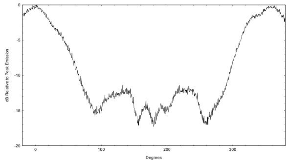
Figure 5-6-1. Example of Directional UWB Antenna Pattern
