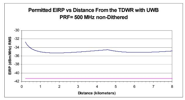
Figure 4-22 Maximum Permitted UWB EIRP for non-Dithered PRF of 500 MHz (UWB Height = 2m).
