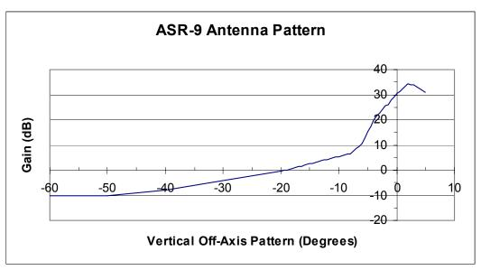
Figure A-6. ASR-9 Vertical Antenna Pattern.
