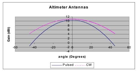
Figure A-7. Altimeter Vertical Antenna Patterns.
