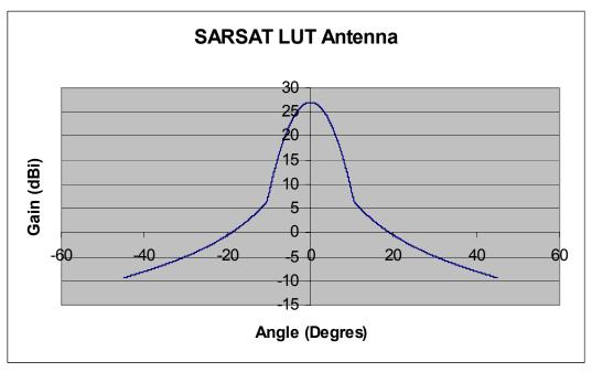
Figure A-13. SARSAT LUT Vertical Antenna Pattern.
