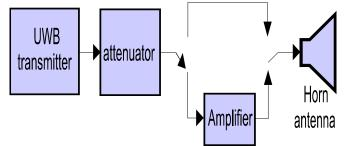
Figure C-1. UWB Pulsar Equipment Configuration.
