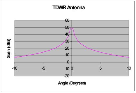
Figure A-14. TDWR Vertical Antenna Pattern.
