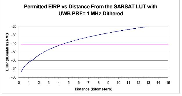
Figure 4-14b. Maximum Permitted UWB EIRP for Dithered PRF of 1 MHz (UWB Height = 2m).
