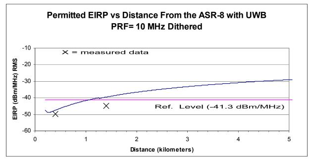
Figure 3-9. Comparison of Measured and Predicted Maximum Permitted EIRP Versus Distance From ASR-8 for 10 MHz Measured Dithered UWB Signal
