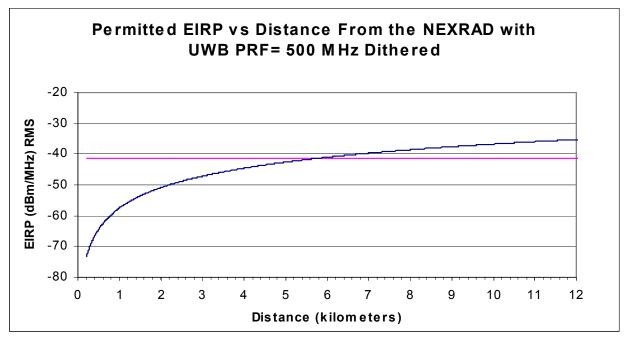
Figure 4-4. Maximum Permitted UWB EIRP for Dithered PRF (UWB Height = 30 m).
