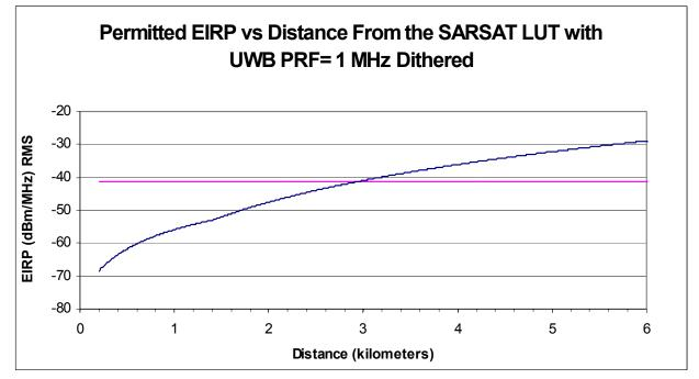
Figure 4-14a. Maximum Permitted UWB EIRP for Dithered PRF of 1 MHz (UWB Height = 2m).
