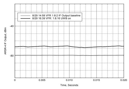
Figure C-4. ARSR-4 IF Output for Baseline Noise Level (UWB signal off) and UWB Signal on for Site # 2 (2.1 km). Peak Detected in 1 MHz Resolution Bandwidth and 10 Hz Video Bandwidth.
