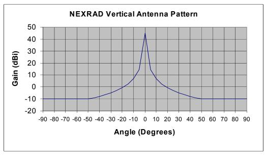
Figure A-2. NEXRAD Vertical Antenna Pattern.
