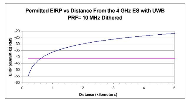
Figure 4-20d. Maximum Permitted UWB EIRP for Dithered PRF of 10 MHz UWB Height = 30m.
