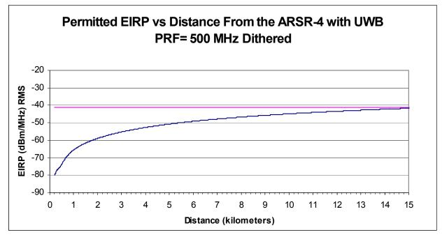
Figure 4-8. Maximum Permitted UWB EIRP for Dithered PRF (UWB Height = 30 m).
