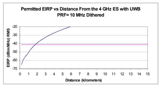
Figure 4-19b. Maximum Permitted UWB EIRP for Dithered PRF of 10 MHz (UWB Height = 2m).
