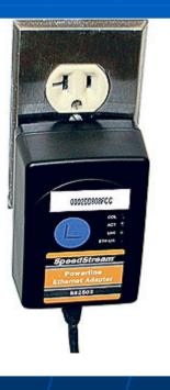
HomePlug Modem can turn an electrical outlet into an Internet connection.
