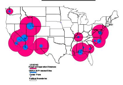
3G Separation Distances at Sites where DoD fixed microwave, tactical radio relay, and aeronautical mobile stations in the 1710 -1755 MHz band will continue operations indefinitely under OBRA '93
