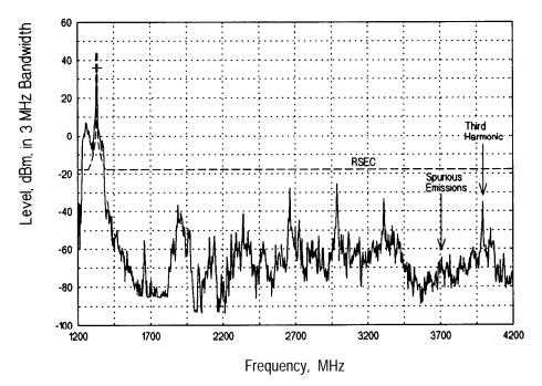
Figure 15. Emission spectrum of a long-range air search radar. Both spurious emissions and third harmonic occur in the 4-GHz band. Third harmonic produced interference to a terrestrial 4-GHz link.
