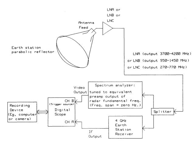
Figure 21. Block diagram for determination of interference coupling mechanism. Characteristics of either front-end overload or radar spurious emissions are observed in coincidence with radar pulses.
