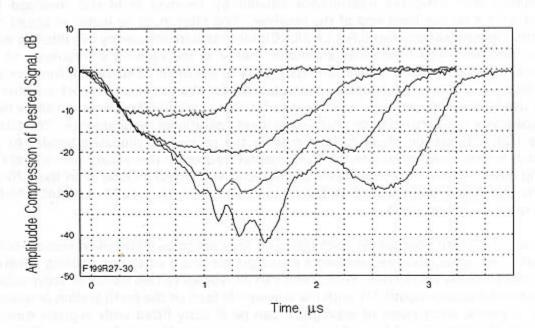
Figure 10. Time domain behavior of LNB #2 at gain compressions of 10, 20, 30 and 40 dB in desired signal at 4000 MHz. Compression created by out-of-band pulses (1-µs pulse width) at 3500 MHz.
