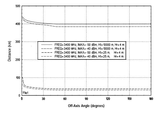
Figure 17. Separation distances required to preclude earth station front-end overload by radar fundamental, as a function of I<sub>max</sub> and antenna height. See text for station parameters.
