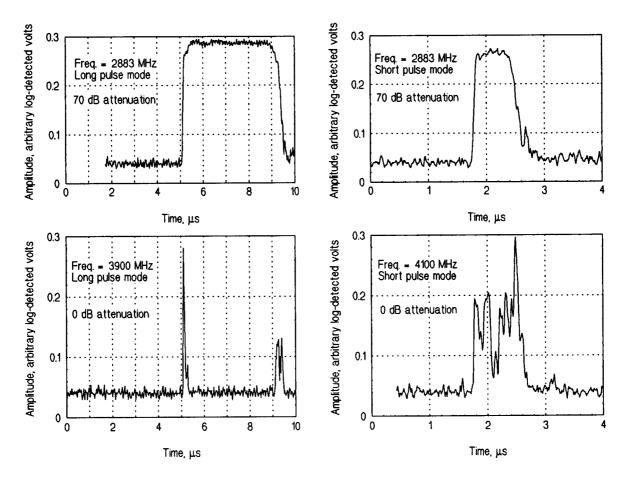
Figure 19. Time waveforms of radar in two pulse modes (long and short) at center frequency (2883 MHz), and at two frequencies in the 3700- to 4200-MHz band. Radiated measurement in 3-MHz bandwidth.
