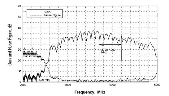
Figure 2. Gain and noise figure of a 4-GHz LNA. Same LNA model has been used in an earth station experiencing RF interference. Y-factor calibration performed with + 18 dB ENR noise diode.
