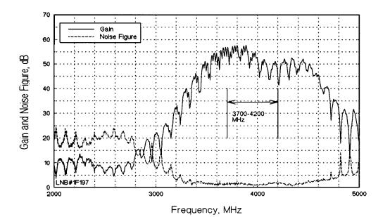
Figure 3. Gain and noise figure of a 4-GHz LNB. Output converted graphically ( $f_{graph} = 5150 \text{ MHz} - f_{output}$ ) to show frequency response. Calibration with + 18 dB ENR noise diode.
