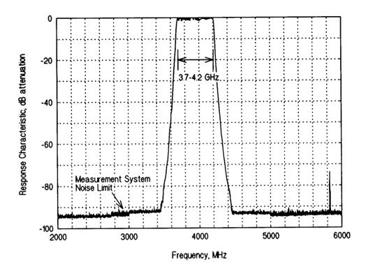
Figure 11. Frequency response curve of a commercially procured 3700-to 4200-MHz bandpass filter of same type as were used to mitigate out-of-band interference to 4-GHz TVRO receivers in south Florida.
