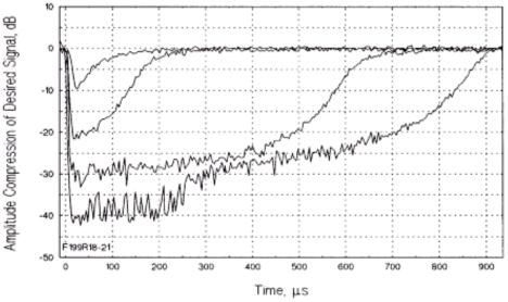
Figure 8. Time domain behavior of LNA at gaiin compression of 10, 20, 30 and 40 dB in desired signal at 4000 MHz. Compression created by out-of-band pulses (1-µs pulse width) at 3500 MHz.
