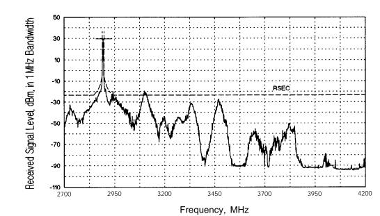
Figure 14. Spectrum of a WSR-74S weather radar, showing spurious emissions in the 3700- to 4200-MHz range. The spurious emissions from this radar caused interference to a 4-GHz terrestrial radio link.
