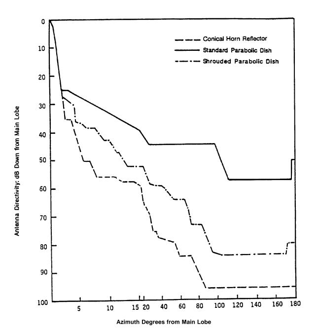
Figure 16. Comparison of directivities for three high-gain antenna types. Shrouded parabolas and conical horns can exhibit higher directivities than ordinary parabolic. Note scale change at 15 degrees.
