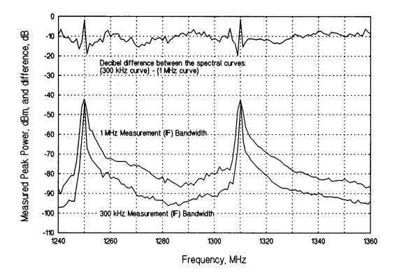
Figure A-2. Measured emission spectra of a radar in two different measurement bandwidths. The center frequency power level does not change, but the spurious emissions change by about 20 log(bandwidth ratio) = 10 dB.
