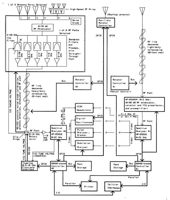
Figure A-1. Block diagram of the NTIA/ITS Radio Spectrum Measurement System (RSMS). The RSMS is a Department of Commerce asset used to assess and resolve radio spectrum occupancy questions and problems.
