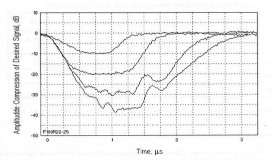
Figure 9. Time domain behavior of LNB #1 at gain compressions of 10, 20, 30 and 40 dB in desired signal at 4000 MHz. Compression created by out-of-band pulses (1-µs pulse width) at 3500 MHz.
