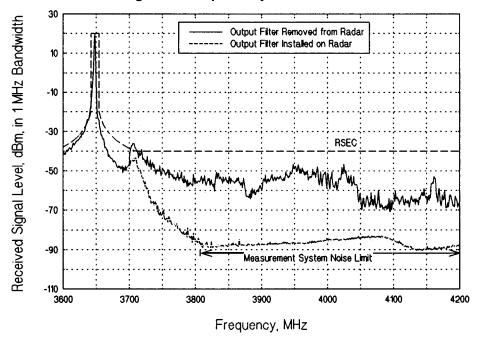
Figure 13. Spectrum of a naval radar showing effect on spectrum when bandpass filter is installed on radar output. Filtered radar output caused front-end overload interference to a TVRO at San Diego, CA.
