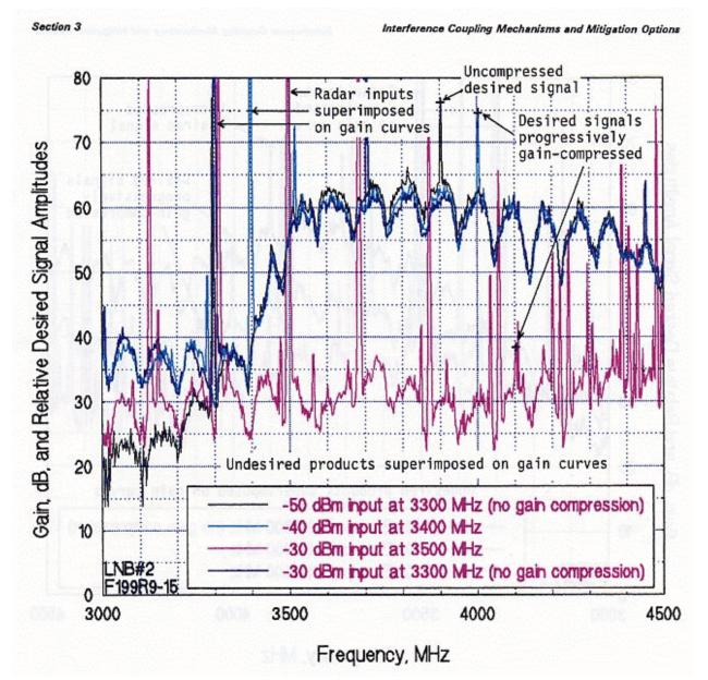
Figure 7. LNB #2 response as a function of simulated radar input. Radar inputs identical to Figures 5-6. Built-in bandpass has decreased susceptibility to overload at input frequencies below 3500 MHz.
