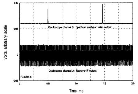
Figure 24. Channels A and B of oscilloscope when test arrangement of Figure 21 is used and radar pulses are not overloading LNA front-end.
