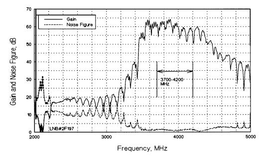
Figure 4. Gain and noise figure of a second 4-GHz LNB, specified by manufacturer as incorporating bandpass filtering. Y-factor calibration performed with + 18 dB ENR noise diode.
