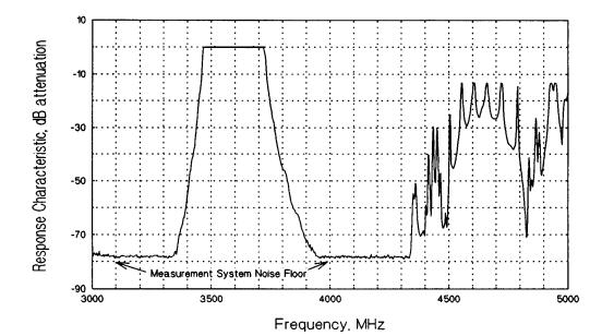
Figure 12. Measured frequency response curve of a bandpass filter installed on naval radar (Figure 13) to suppress spurious emissions and enhance electromagnetic compatibility with 4-GHz receivers.
