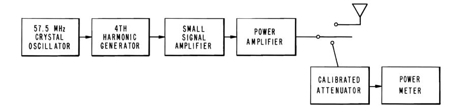
Figure 15. Transmitter block diagram
