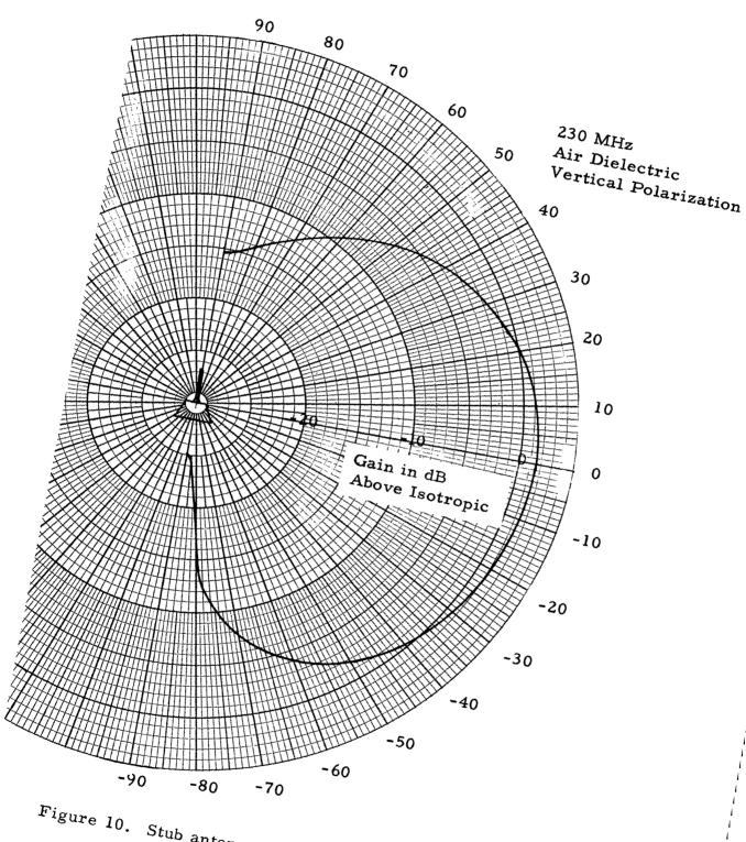
Figure 10. Stub antenna vertical pattern for 230  $_{
