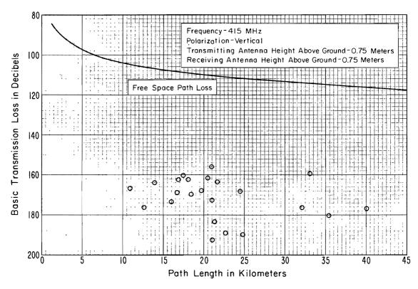
Figure 19. Idaho area radio path loss at 415.9 MHz
