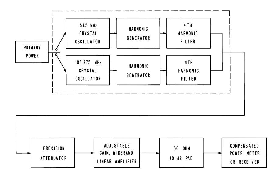
Figure 14. Signal generator block diagram
