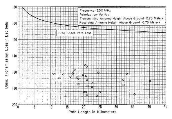
Figure 18. Idaho area radio path loss at 230 MHz
