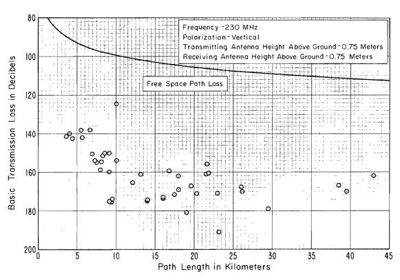
Figure 16. Wyoming area radio path loss at 230 MHz
