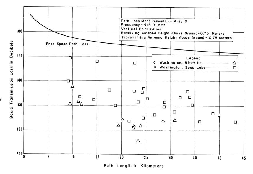
Figure 26. Basic transmission loss Washington intra-area comparison
