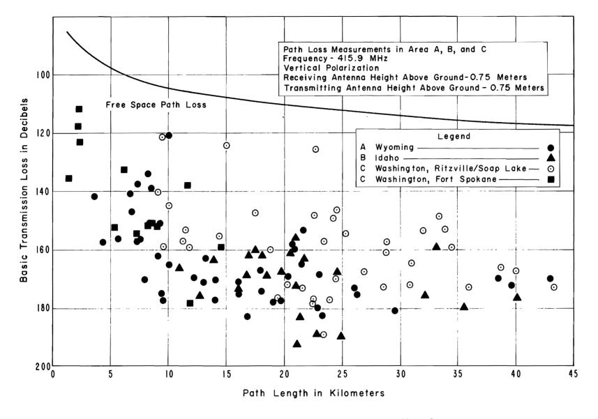
Figure 25. Basic transmission loss for all paths.
