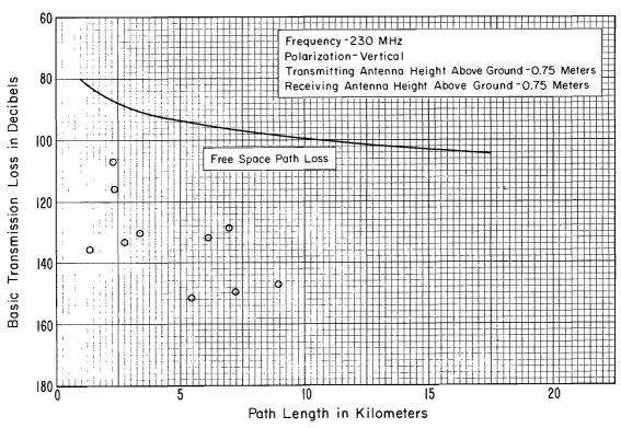
Figure 22. Washington area (Fort Spokane) radio path loss at 230 MHz
