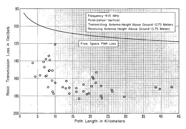
Figure 17. Wyoming area radio path loss at 415.9 MHz
