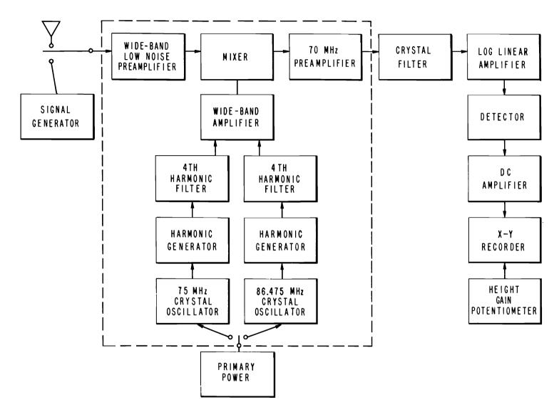
Figure 11. Receiver block diagram.
