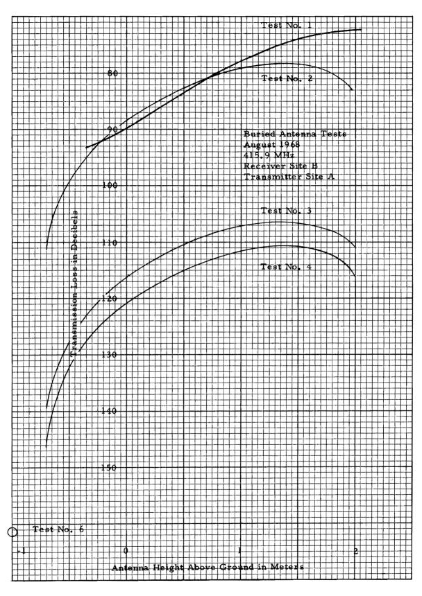
Figure 47. Buried antenna test results for tests 1, 2, 3, 4, and 6.
