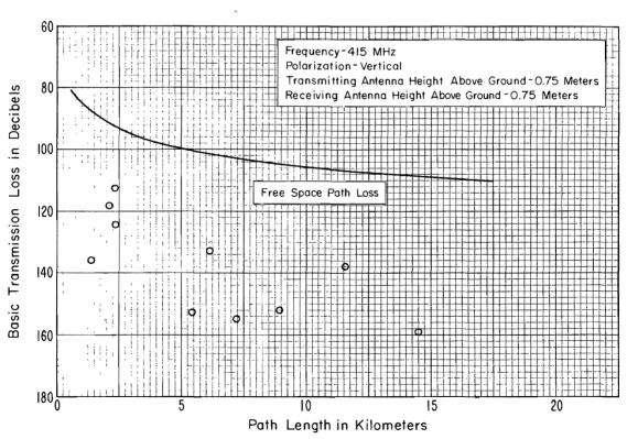
Figure 23. Washington area (Fort Spokane) radio path loss at 415.9 MHz
