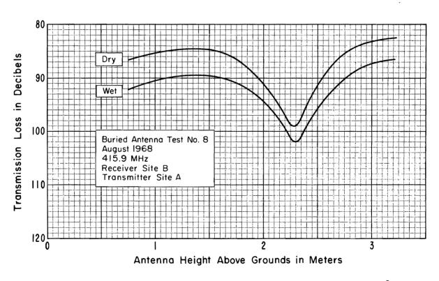
Figure 50. Buried antenna test results for test no. 8.
