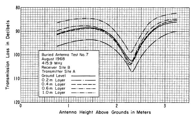
Figure 49. Buried antenna test results for test no. 7.
