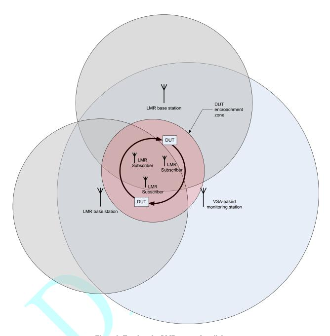
Figure 9: Topology for LMR system downlink test
