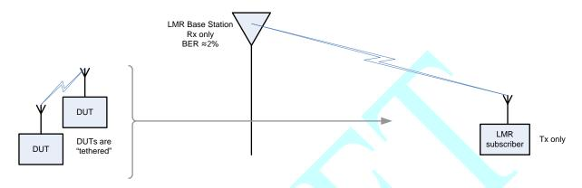
Figure 7: Topology for LMR system uplink test
