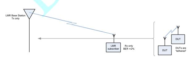
Figure 4: Topology for LMR system downlink test
