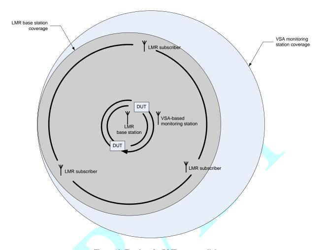
Figure 10: Topology for LMR system uplink test
