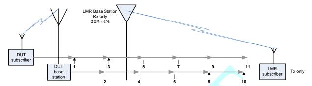
Figure 8: Topology for LMR system uplink test for DUTs with fixed base stations
