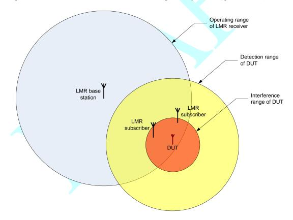
Figure 2: Typical LMR downlink hidden node scenario
