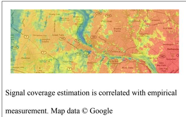
coverage models with empirical measurement and presents a highly accurate digital representation of real-world and predicted spectrum environments.
