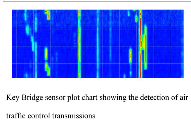
commercial air-to-ground, ground-to-air and ground-to-ground communications, scanning a 2 MHz span at 10 times per second with high precision.
