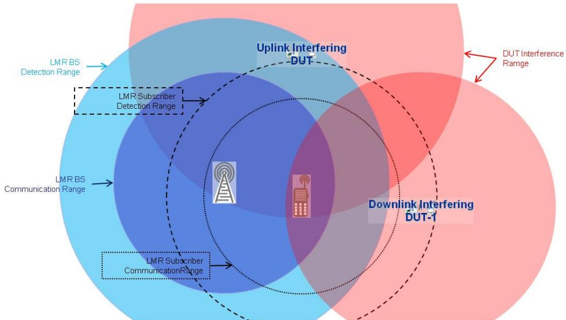
Figure 3: Illustration downlink and uplink hidden nodes.
