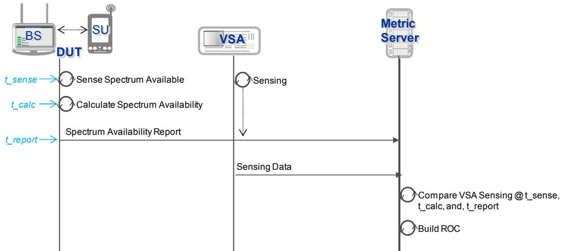
Figure 1: Illustration of Phase II channel availability check.
