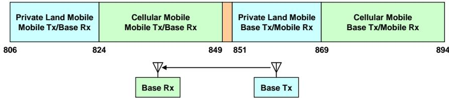
Figure 10 – Base-to-base interference in the 800 MHz band
