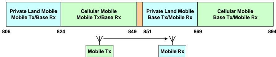
Figure 11 – Mobile-to-mobile interference in the 800 MHz band
