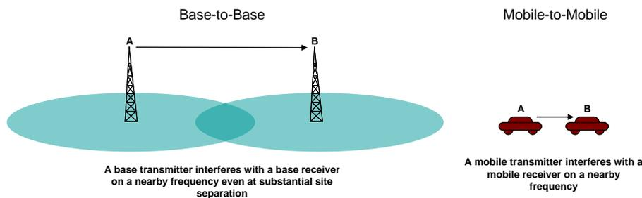
Figure 6 – Interference paths in unpaired spectrum.
