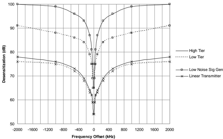
Figure 3 – Desensitization curves for typical land-mobile radio receivers
