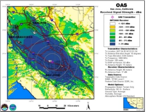
OAS, Antenna Elevation Angle: 10°, Transmitter Power: 100 W, IMT-2000 Base Station
