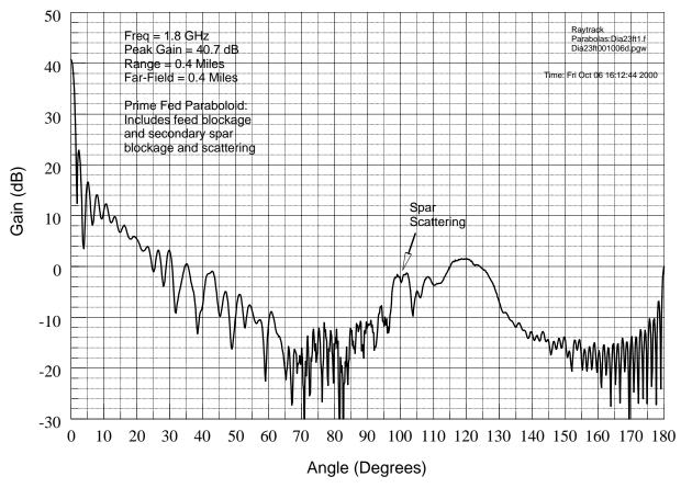
Datron 23' Antenna: Gain vs. Angle
