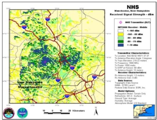
NHS-DLT, Antenna Elevation Angle: 3°, Transmitter Power: 1,000 W, IMT-2000 Mobile Station
