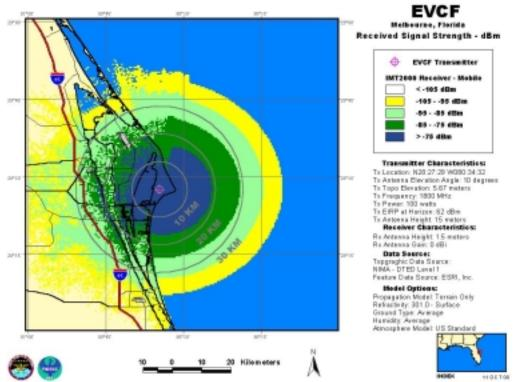
EVCF, Antenna Elevation Angle: 10°, Transmitter Power: 100 W, IMT-2000 Mobile Station
