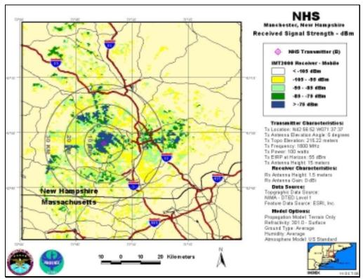
NHS-B, Antenna Elevation Angle: 5°, Transmitter Power: 100 W, IMT-2000 Mobile Station
