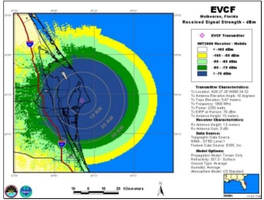
EVCF, Antenna Elevation Angle: 10°, Transmitter Power: 2,250 W, IMT-2000 Mobile Station
