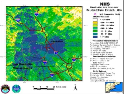
NHS-DLT, Antenna Elevation Angle: 3°, Transmitter Power: 100 W, IMT-2000 Base Station
