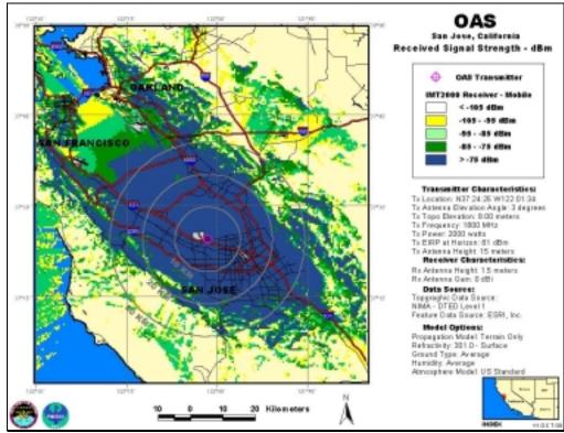
OAS, Antenna Elevation Angle: 3°, Transmitter Power: 2,000 W, IMT-2000 Mobile Station
