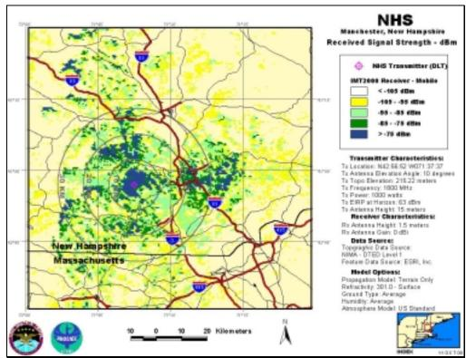
NHS-DLT, Antenna Elevation Angle: 10°, Transmitter Power: 1,000 W, IMT-2000 Mobile Station
