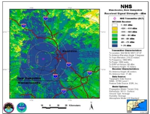
NHS-DLT, Antenna Elevation Angle: 3°, Transmitter Power: 1,000 W, IMT-2000 Base Station
