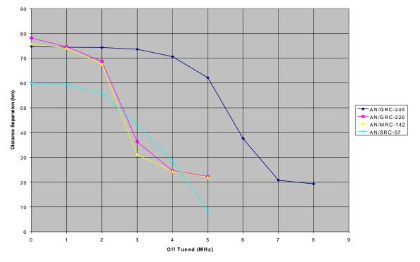
Figure C-1. Frequency-Distance Separation for CDMA-WB to TRR
