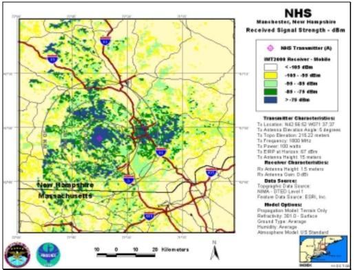
NHS-A, Antenna Elevation Angle: 5°, Transmitter Power: 100 W, IMT-2000 Mobile Station
