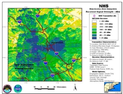
NHS-B, Antenna Elevation Angle: 10°, Transmitter Power: 100 W, IMT-2000 Base Station
