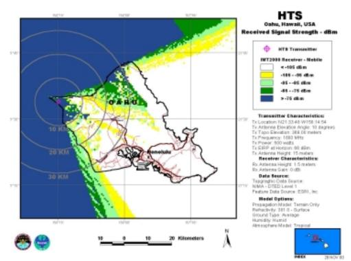
HTS, Antenna Elevation Angle: 10°, Transmitter Power: 500 W, IMT-2000 Mobile Station
