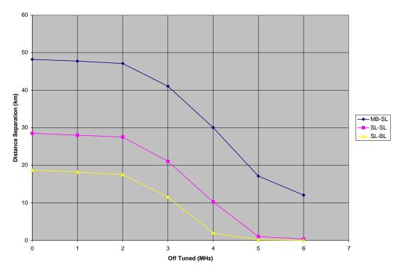
Figure C-10. Frequency-Distance Separation for a TRR to AN/TRC-170
