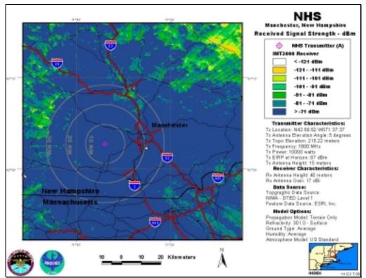
NHS-A, Antenna Elevation Angle: 5°, Transmitter Power: 10,000 W, IMT-2000 Base Station
