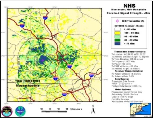
NHS-A, Antenna Elevation Angle: 10°, Transmitter Power: 100 W, IMT-2000 Mobile Station
