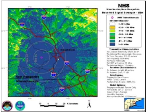
NHS-A, Antenna Elevation Angle: 3°, Transmitter Power: 100 W, IMT-2000 Base Station
