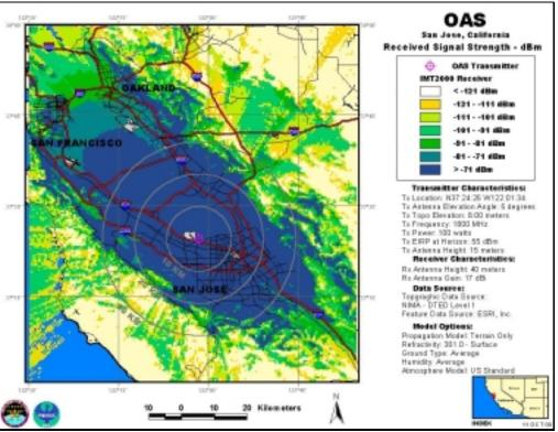
OAS, Antenna Elevation Angle: 5°, Transmitter Power: 100 W, IMT-2000 Base Station
