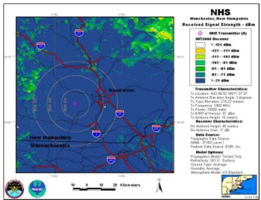
NHS-A, Antenna Elevation Angle: 3°, Transmitter Power: 10,0000 W, IMT-2000 Base Station
