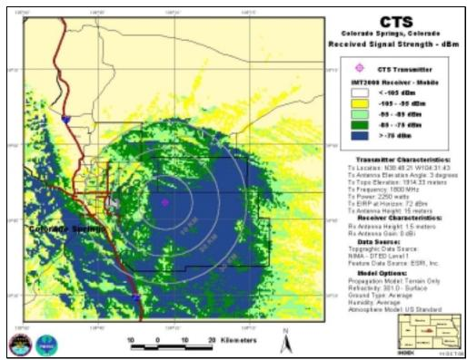
CTS, Antenna Elevation Angle: 3°, Transmitter Power: 2,250 W, IMT-2000 Mobile Station
