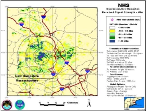
NHS-DLT, Antenna Elevation Angle: 10°, Transmitter Power: 100 W, IMT-2000 Mobile Station
