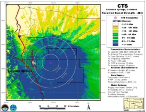
CTS, Antenna Elevation Angle: 5°, Transmitter Power: 100 W, IMT-2000 Base Station
