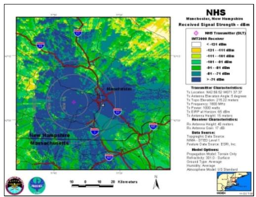
NHS-DLT, Antenna Elevation Angle: 5°, Transmitter Power: 1,000 W, IMT-2000 Base Station
