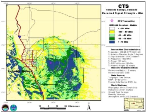
CTS, Antenna Elevation Angle: 3°, Transmitter Power: 100 W, IMT-2000 Mobile Station
