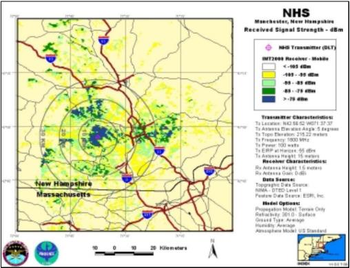
NHS-DLT, Antenna Elevation Angle: 5°, Transmitter Power: 100 W, IMT-2000 Mobile Station
