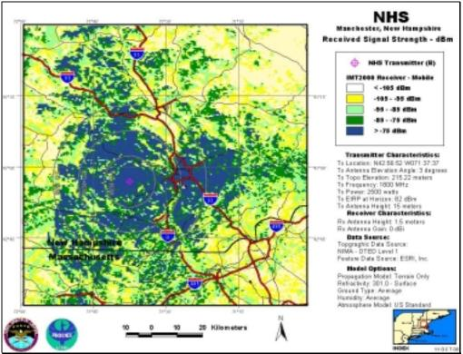
NHS-B, Antenna Elevation Angle: 3°, Transmitter Power: 2,500 W, IMT-2000 Mobile Station
