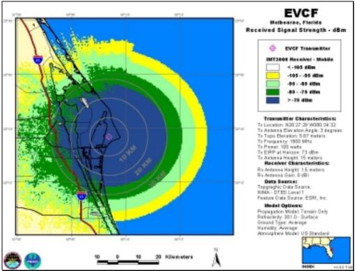
EVCF, Antenna Elevation Angle: 3°, Transmitter Power: 100 W, IMT-2000 Mobile Station
