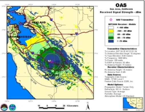
OAS, Antenna Elevation Angle: 10°, Transmitter Power: 100 W, IMT-2000 Mobile Station
