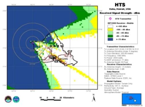
HTS, Antenna Elevation Angle: 5°, Transmitter Power: 2000 W, IMT-2000 Mobile Station
