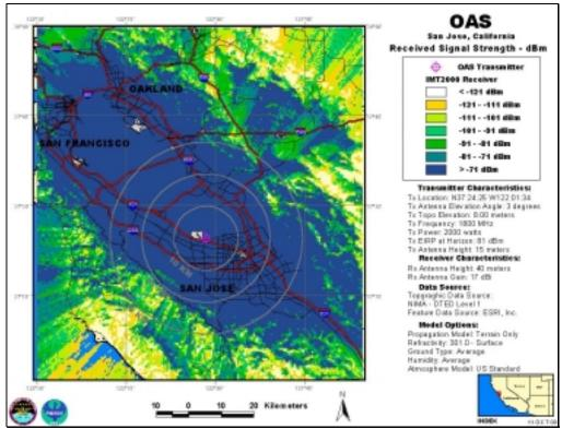
OAS, Antenna Elevation Angle: 3°, Transmitter Power: 2,000 W, IMT-2000 Base Station
