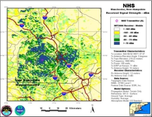
NHS-A, Antenna Elevation Angle: 3°, Transmitter Power: 100 W, IMT-2000 Mobile Station
