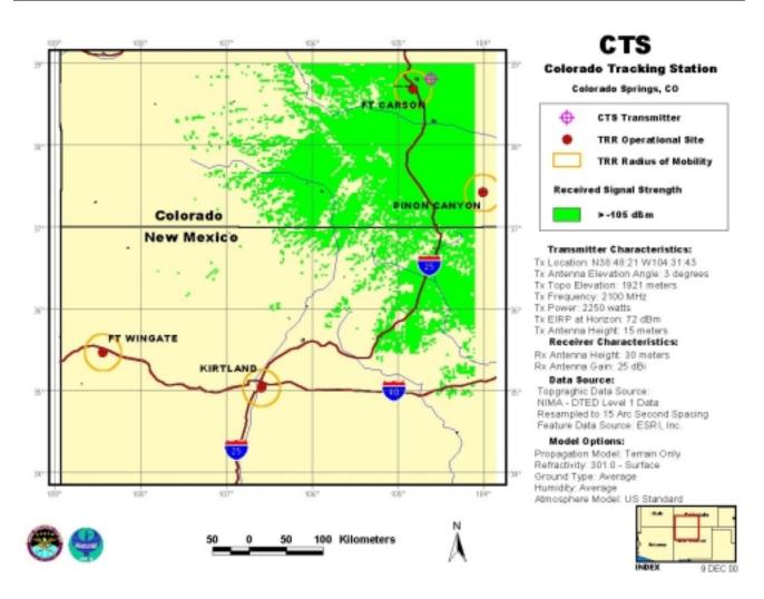
Figure C-6. Plot of CTS SGLS Interference to TRR Receivers
