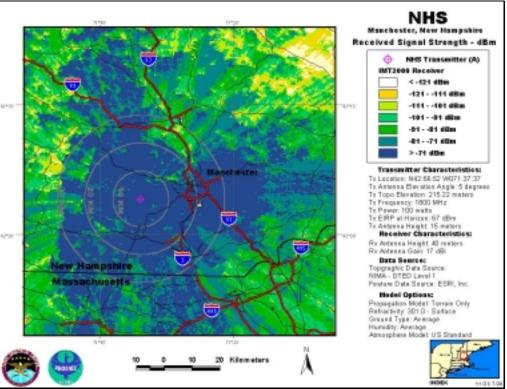
NHS-A, Antenna Elevation Angle: 5°, Transmitter Power: 100 W, IMT-2000 Base Station
