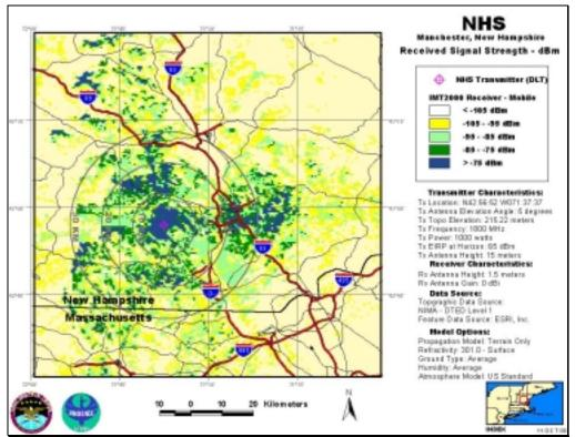
NHS-DLT, Antenna Elevation Angle: 5°, Transmitter Power: 1,000 W, IMT-2000 Mobile Station
