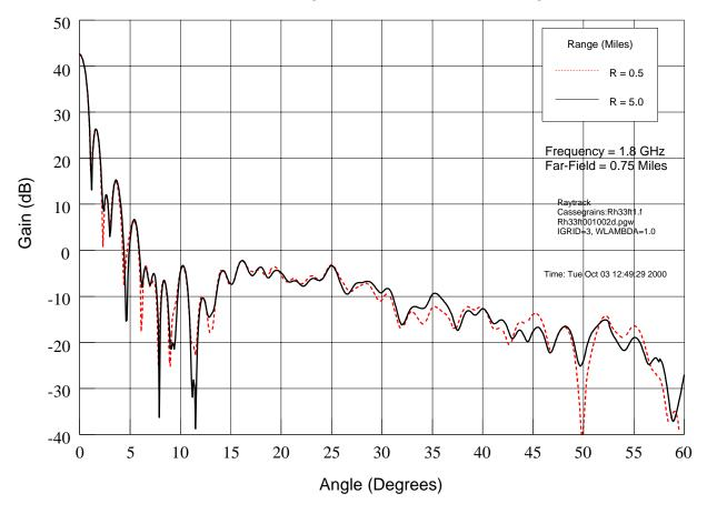
33 Ft. Cassegrain Antenna: Gain vs. Angle
