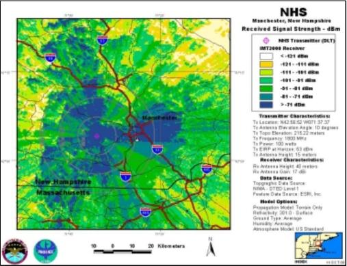
NHS-DLT, Antenna Elevation Angle: 10°, Transmitter Power: 100 W, IMT-2000 Base Station
