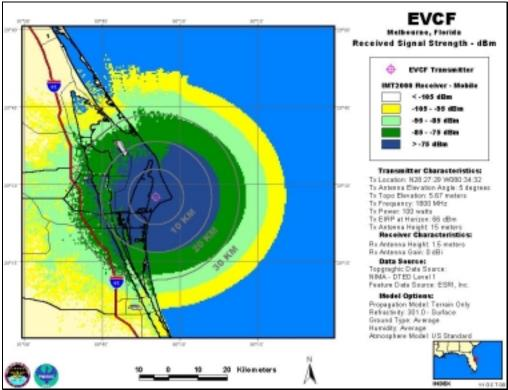
EVCF, Antenna Elevation Angle: 5°, Transmitter Power: 100 W, IMT-2000 Mobile Station
