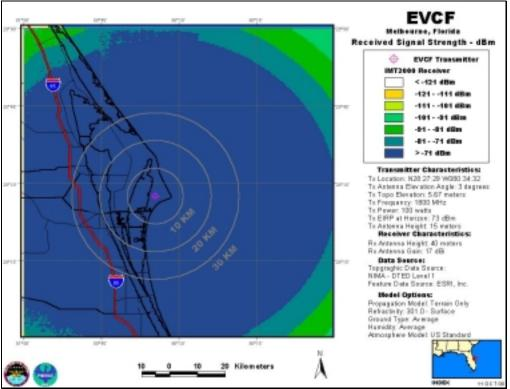
EVCF, Antenna Elevation Angle: 3°, Transmitter Power: 100 W, IMT-2000 Base Station
