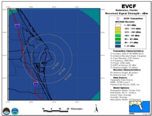
EVCF, Antenna Elevation Angle: 3°, Transmitter Power: 2,250 W, IMT-2000 Base Station
