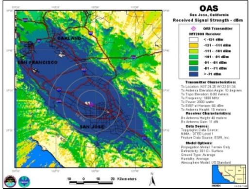
OAS, Antenna Elevation Angle: 10°, Transmitter Power: 2,000 W, IMT-2000 Base Station
