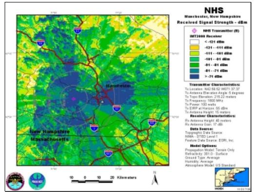
NHS-B, Antenna Elevation Angle: 5°, Transmitter Power: 100 W, IMT-2000 Base Station
