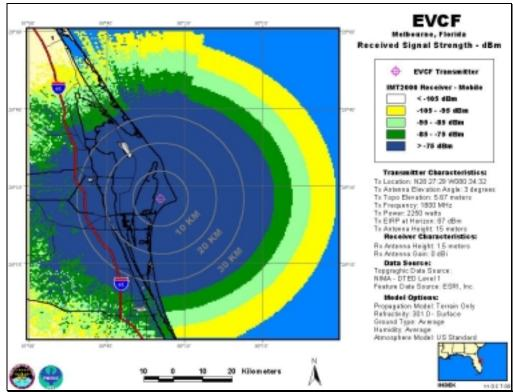
EVCF, Antenna Elevation Angle: 3°, Transmitter Power: 2,250 W, IMT-2000 Mobile Station
