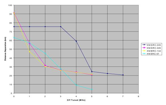
Figure C-2. Frequency-Distance Separation for IMT-2000 GSM to TRR
