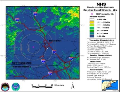
NHS-B, Antenna Elevation Angle: 3°, Transmitter Power: 2,500 W, IMT-2000 Base Station
