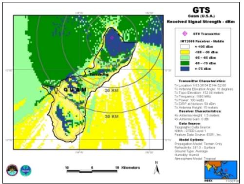
GTS, Antenna Elevation Angle: 10°, Transmitter Power: 100 W, IMT-2000 Mobile Station
