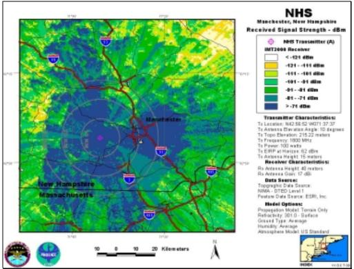
NHS-A, Antenna Elevation Angle: 10°, Transmitter Power: 100 W, IMT-2000 Base Station
