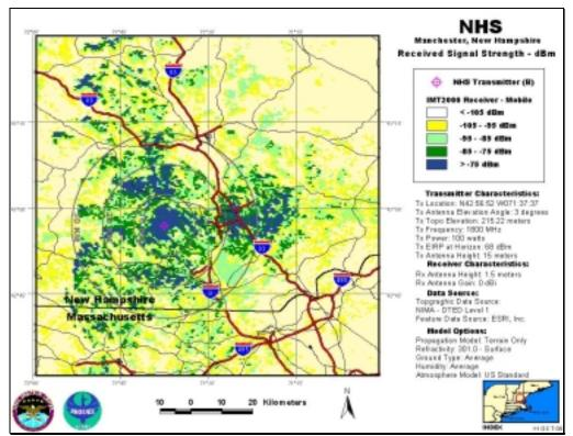
NHS-B, Antenna Elevation Angle: 3°, Transmitter Power: 100 W, IMT-2000 Mobile Station
