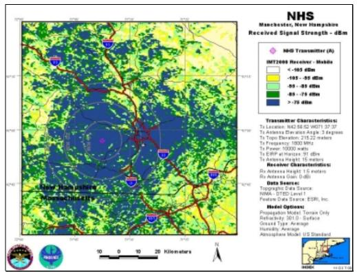
NHS-A, Antenna Elevation Angle: 3°, Transmitter Power: 10,000 W, IMT-2000 Mobile Station
