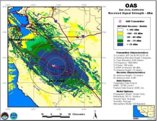
OAS, Antenna Elevation Angle: 3°, Transmitter Power: 100 W, IMT-2000 Mobile Station
