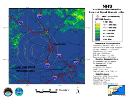
Figure B-6. NHS-A, Antenna Elevation Angle: 3°, Transmitter Power: 10,000 W, IMT-2000 Base Station
