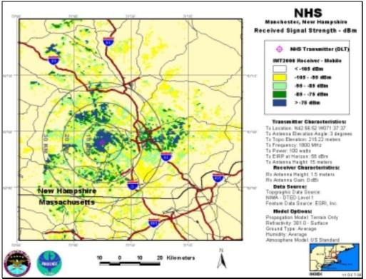
NHS-DLT, Antenna Elevation Angle: 3°, Transmitter Power: 100 W, IMT-2000 Mobile Station
