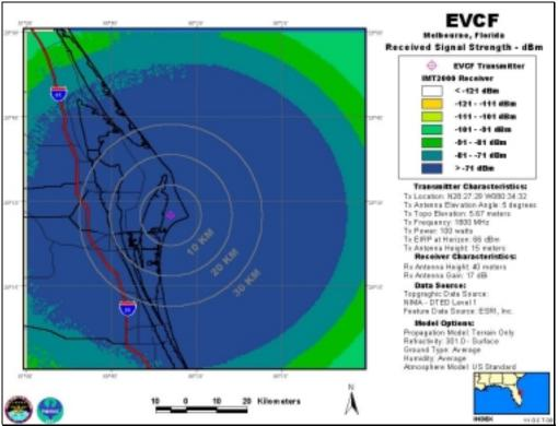
EVCF, Antenna Elevation Angle: 5°, Transmitter Power: 100 W, IMT-2000 Base Station
