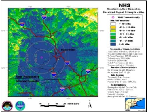
NHS-B, Antenna Elevation Angle: 5°, Transmitter Power: 2,500 W, IMT-2000 Base Station
