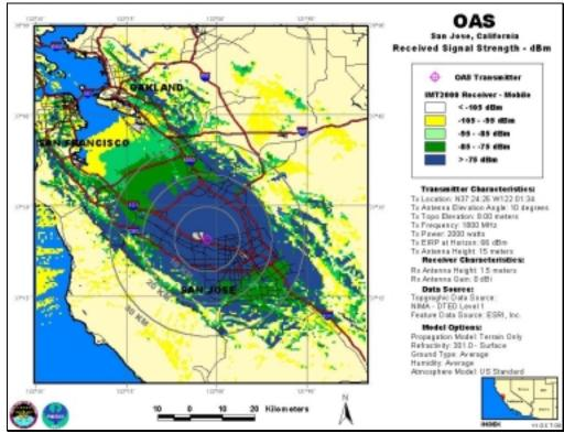
OAS, Antenna Elevation Angle: 10°, Transmitter Power: 2,000 W, IMT-2000 Mobile Station
