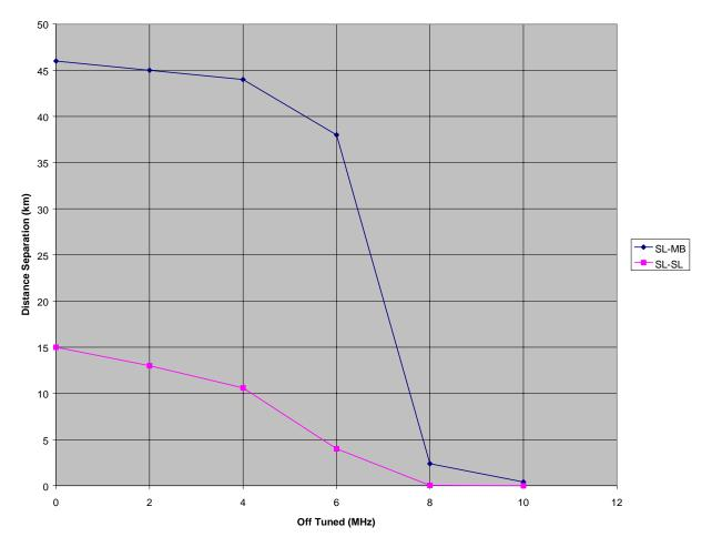
Figure C-11. Frequency-Distance Separation for AN/GRC-222 to a TRR
