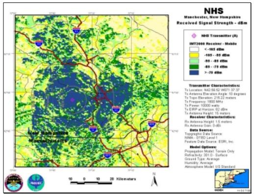
NHS-A, Antenna Elevation Angle: 10°, Transmitter Power: 10,000 W, IMT-2000 Mobile Station
