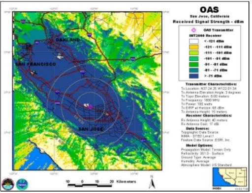
OAS, Antenna Elevation Angle: 3°, Transmitter Power: 100 W, IMT-2000 Base Station
