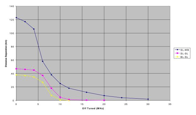
Figure C-9. Frequency-Distance Separation for AN/TRC-170 to a TRR
