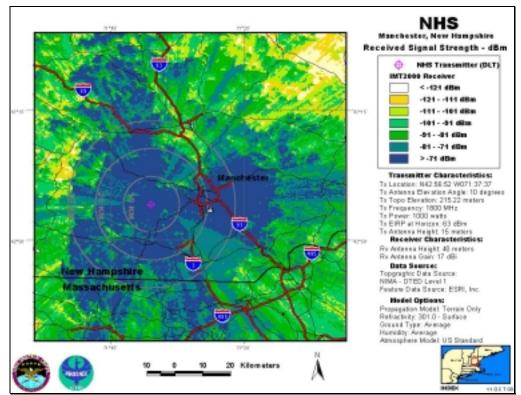
NHS-DLT, Antenna Elevation Angle: 10°, Transmitter Power: 1,000 W, IMT-2000 Base Station
