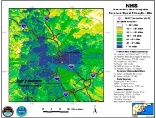
NHS-DLT, Antenna Elevation Angle: 5°, Transmitter Power: 100 W, IMT-2000 Base Station
