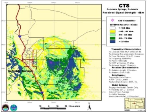
CTS, Antenna Elevation Angle: 5°, Transmitter Power: 100 W, IMT-2000 Mobile Station
