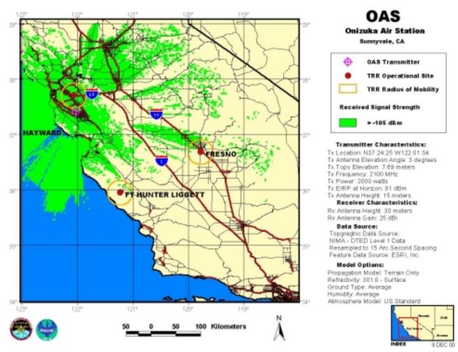
Figure C-8. Plot of OAS SGLS Interference to TRR Receivers
