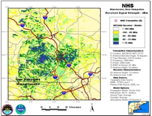
NHS-B, Antenna Elevation Angle: 10°, Transmitter Power: 2,500 W, IMT-2000 Mobile Station
