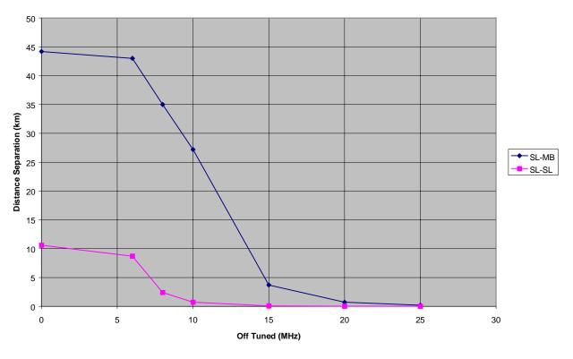
Frequency-Distance Separation for AN/GRC-245 to AN/GRC-222
