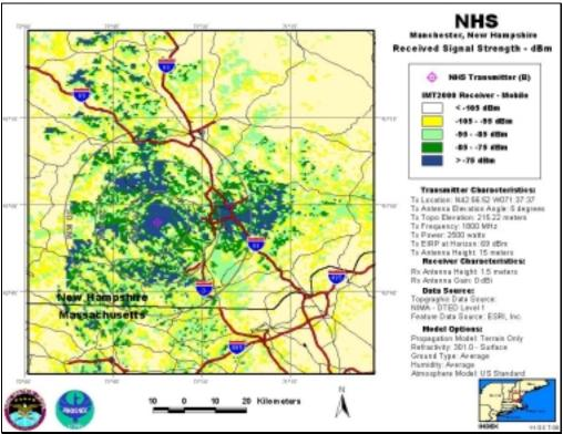
NHS-B, Antenna Elevation Angle: 5°, Transmitter Power: 2,500 W, IMT-2000 Mobile Station
