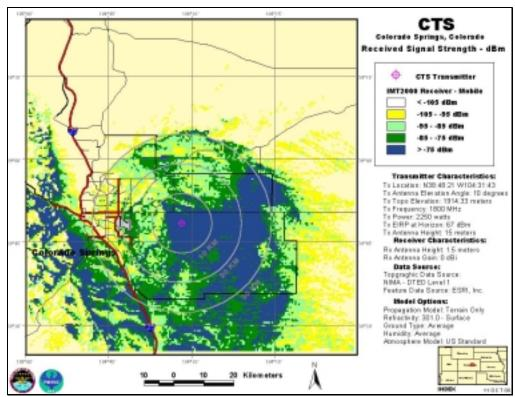
CTS, Antenna Elevation Angle: 10°, Transmitter Power: 2,250 W, IMT-2000 Mobile Station
