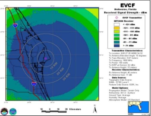
EVCF, Antenna Elevation Angle: 10°, Transmitter Power: 100 W, IMT-2000 Base Station
