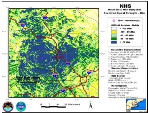
NHS-A, Antenna Elevation Angle: 5°, Transmitter Power: 10,000 W, IMT-2000 Mobile Station
