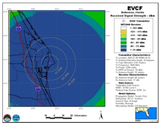
EVCF, Antenna Elevation Angle: 10°, Transmitter Power: 2,250 W, IMT-2000 Base Station
