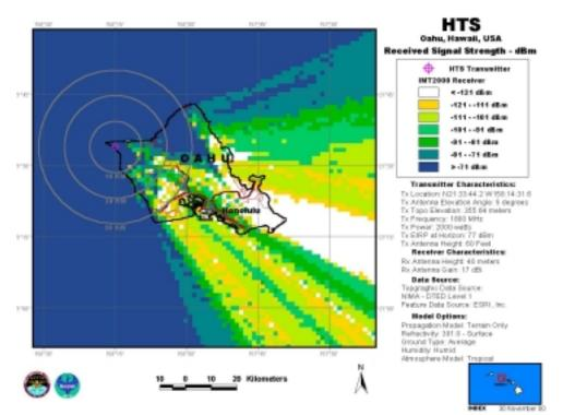
HTS, Antenna Elevation Angle: 5°, Transmitter Power: 2000 W, IMT-2000 Base Station
