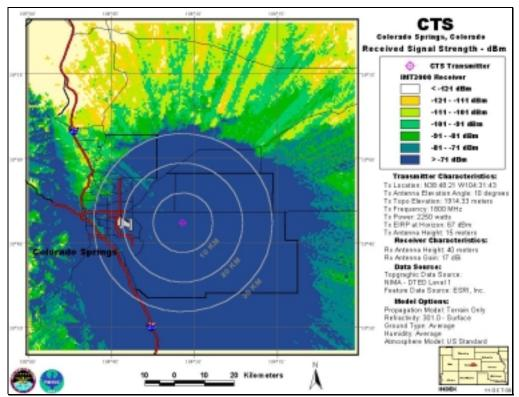
CTS, Antenna Elevation Angle: 10°, Transmitter Power: 2,250 W, IMT-2000 Base Station
