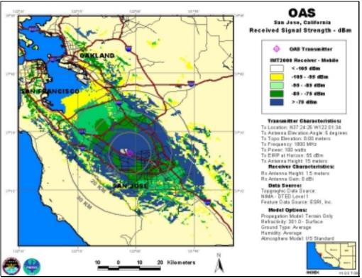
OAS, Antenna Elevation Angle: 5°, Transmitter Power: 100 W, IMT-2000 Mobile Station
