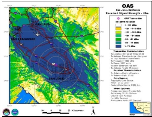
OAS, Antenna Elevation Angle: 5°, Transmitter Power: 2,000 W, IMT-2000 Base Station
