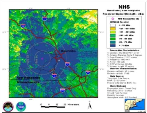
NHS-B, Antenna Elevation Angle: 3°, Transmitter Power: 100 W, IMT-2000 Base Station
