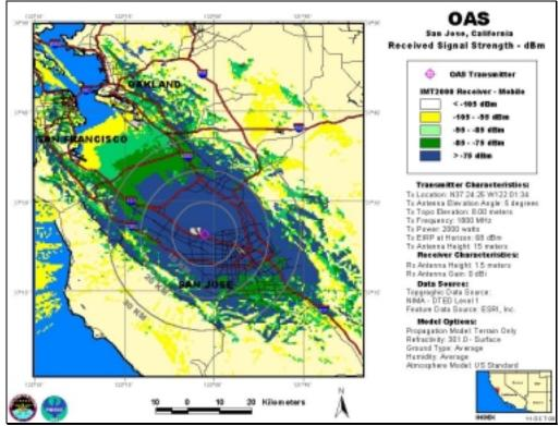
OAS, Antenna Elevation Angle: 5°, Transmitter Power: 2,000 W, IMT-2000 Mobile Station
