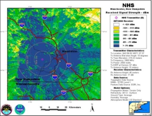
NHS-B, Antenna Elevation Angle: 10°, Transmitter Power: 2,500 W, IMT-2000 Base Station
