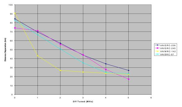
Figure C-4. Frequency-Distance Separation for TRR to GSM
