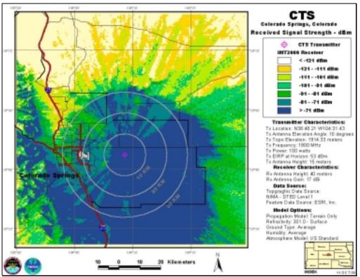
CTS, Antenna Elevation Angle: 10°, Transmitter Power: 100 W, IMT-2000 Base Station
