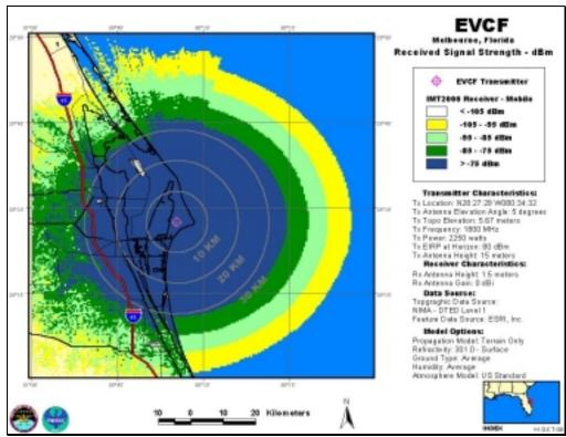
EVCF, Antenna Elevation Angle: 5°, Transmitter Power: 2,250 W, IMT-2000 Mobile Station
