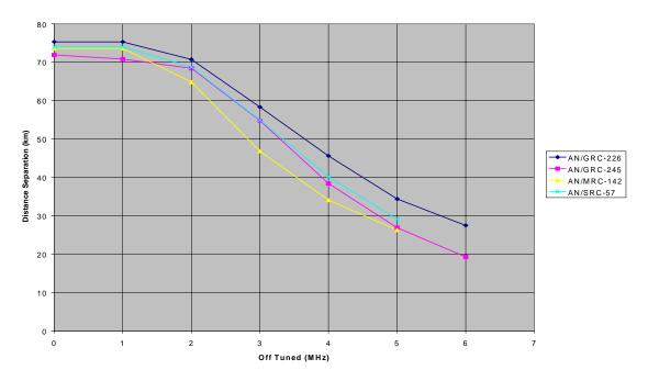
Figure C-3. Frequency-Distance Separation for TRR to CDMA-WB
