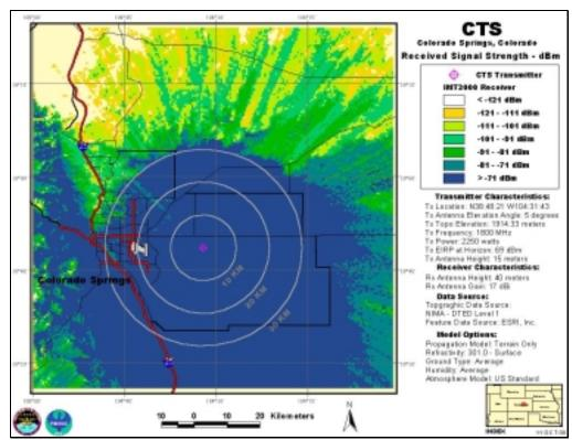
CTS, Antenna Elevation Angle: 5°, Transmitter Power: 2,250 W, IMT-2000 Base Station
