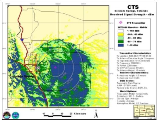
CTS, Antenna Elevation Angle: 5°, Transmitter Power: 2,250 W, IMT-2000 Mobile Station
