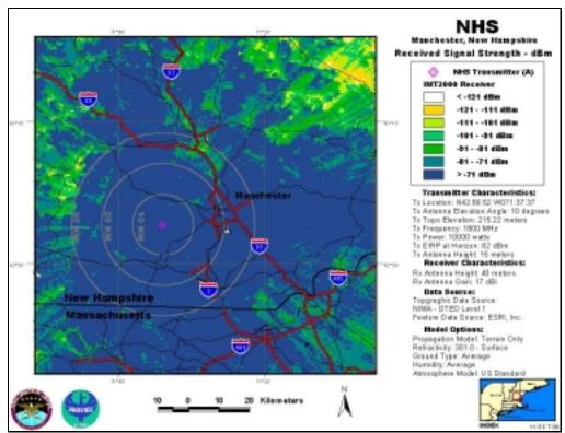
NHS-A, Antenna Elevation Angle: 10°, Transmitter Power: 10,000 W, IMT-2000 Base Station
