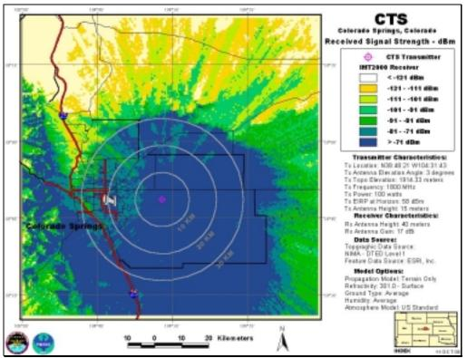
CTS, Antenna Elevation Angle: 3°, Transmitter Power: 100 W, IMT-2000 Base Station
