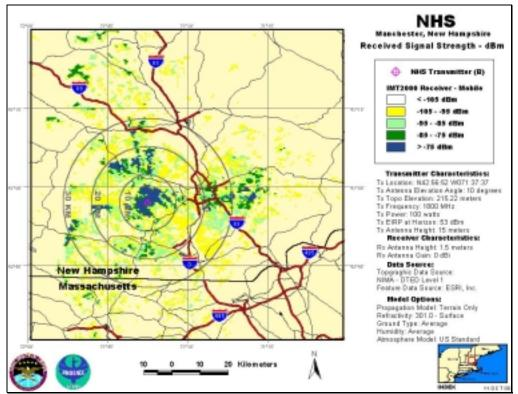
NHS-B, Antenna Elevation Angle: 10°, Transmitter Power: 100 W, IMT-2000 Mobile Station
