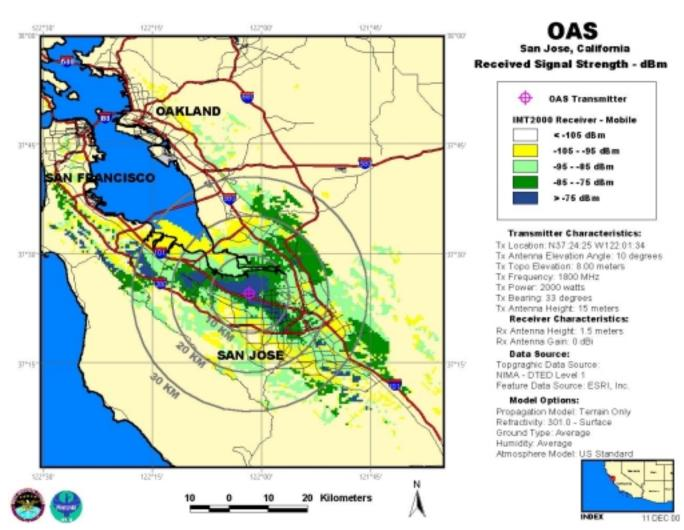
Figure B-14. OAS, Antenna Elevation Angle: 10°, Azimuth 33°, Transmitter Power: 2000 W, IMT-2000 Mobile Station
