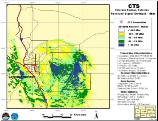
CTS, Antenna Elevation Angle: 10°, Transmitter Power: 100 W, IMT-2000 Mobile Station
