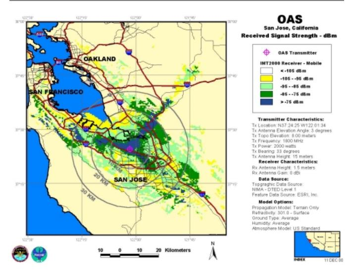
Figure B-13. OAS, Antenna Elevation Angle: 3°, Azimuth 33°, Transmitter Power: 2000 W, IMT-2000 Mobile Station
