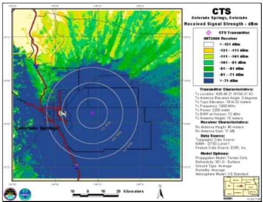
CTS, Antenna Elevation Angle: 3°, Transmitter Power: 2,250 W, IMT-2000 Base Station
