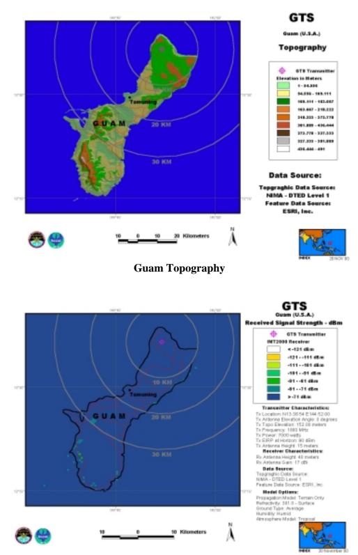
GTS, Antenna Elevation Angle: 3°, Transmitter Power: 7000 W, IMT-2000 Base Station
