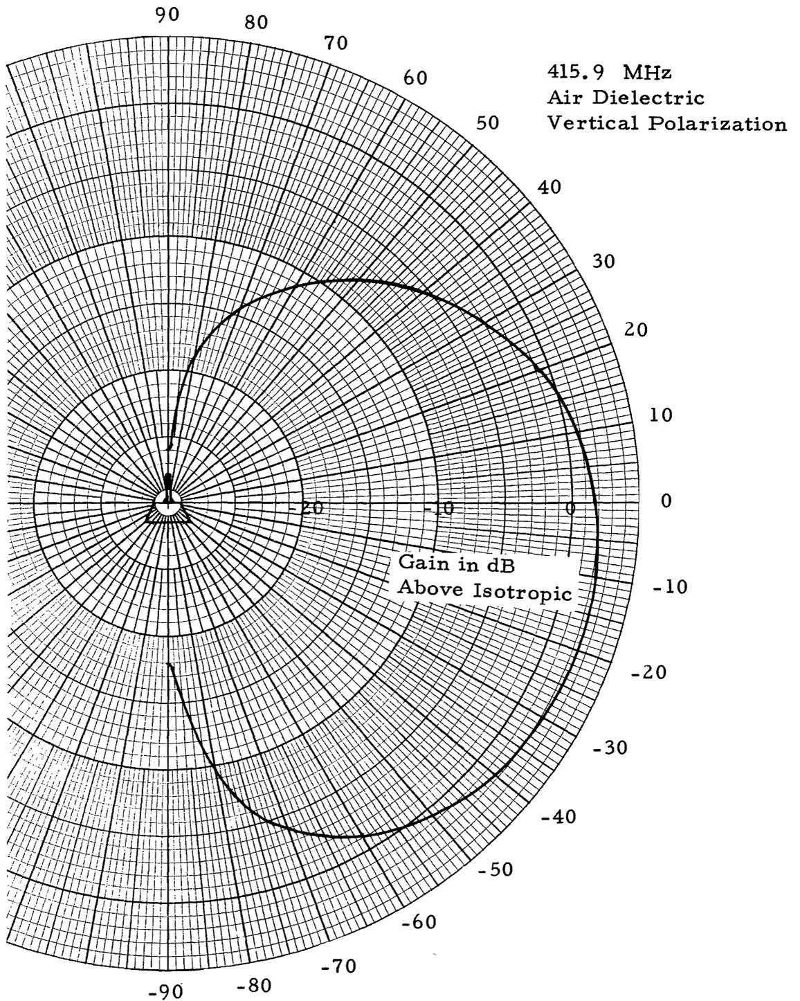
Figure 9. Stub antenna vertical pattern for 415.9 MHz
