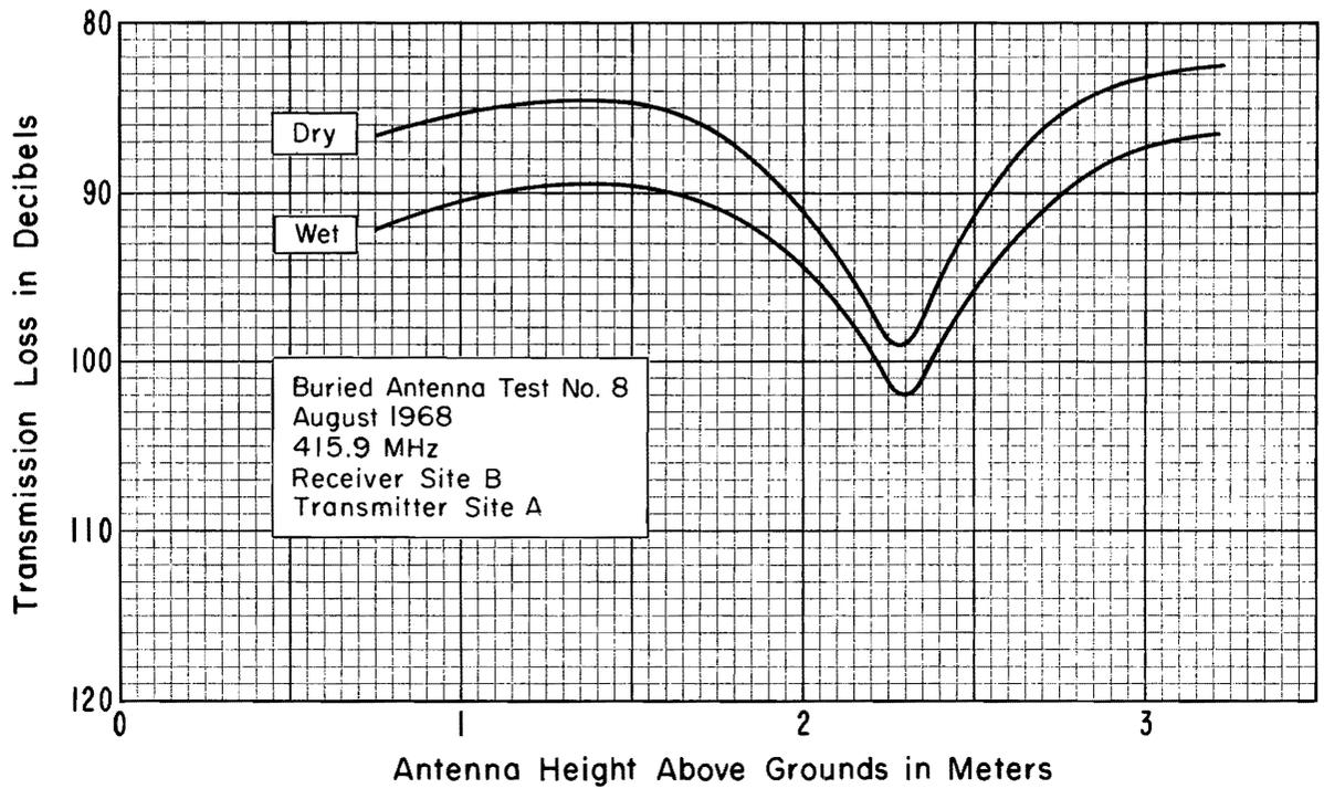
Figure 50. Buried antenna test results for test no. 8.
