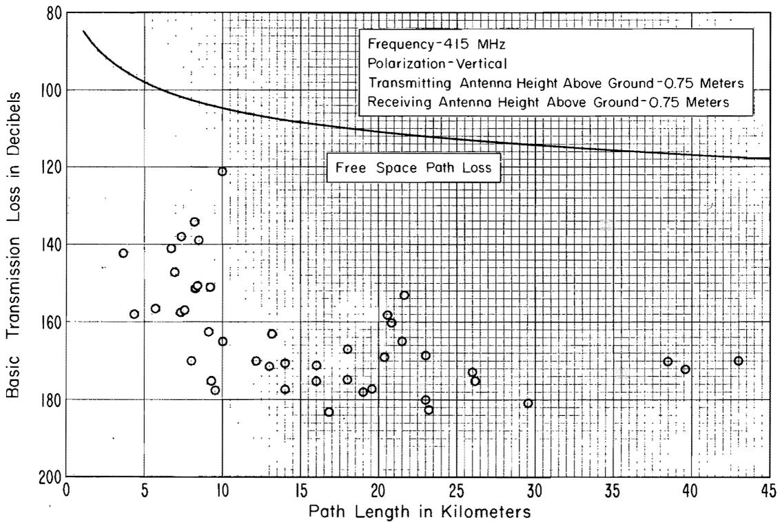
Figure 17. Wyoming area radio path loss at 415.9 MHz
