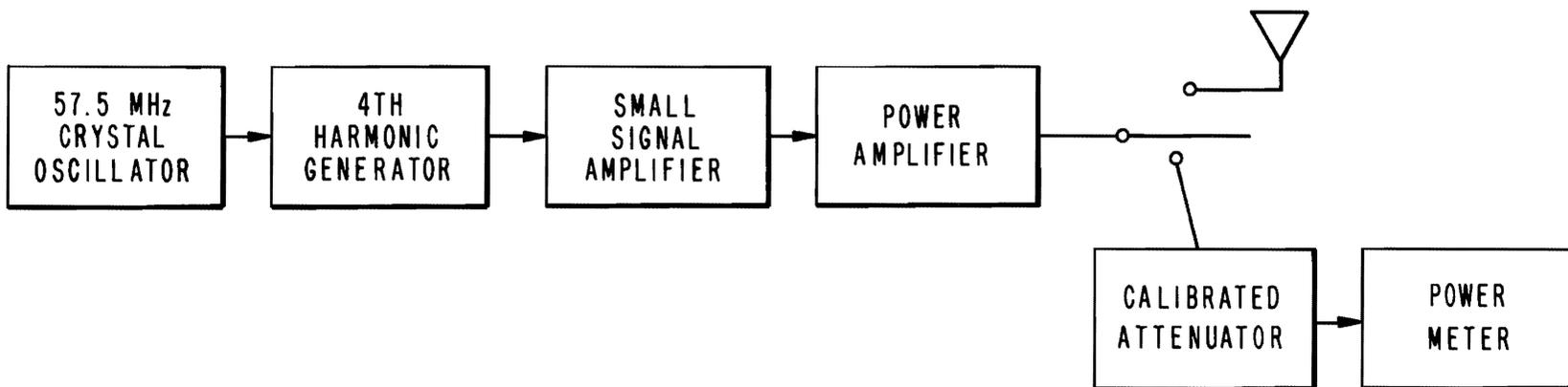
Figure 15. Transmitter block diagram
