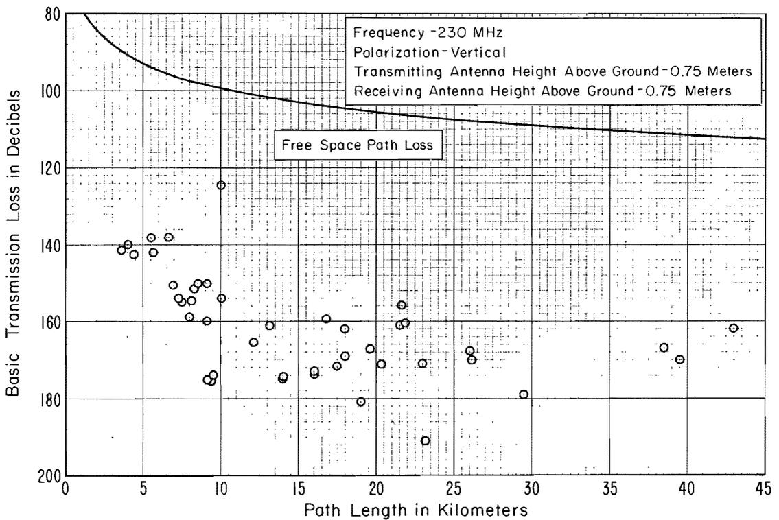
Figure 16. Wyoming area radio path loss at 230 MHz
