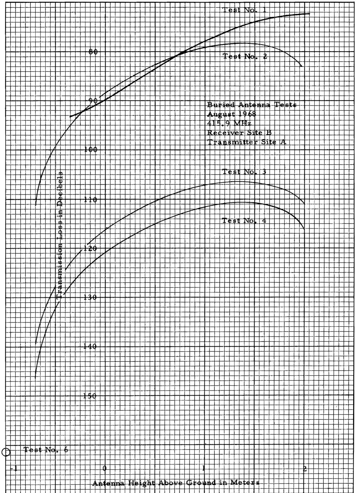
Figure 47. Buried antenna test results for tests 1, 2, 3, 4, and 6.
