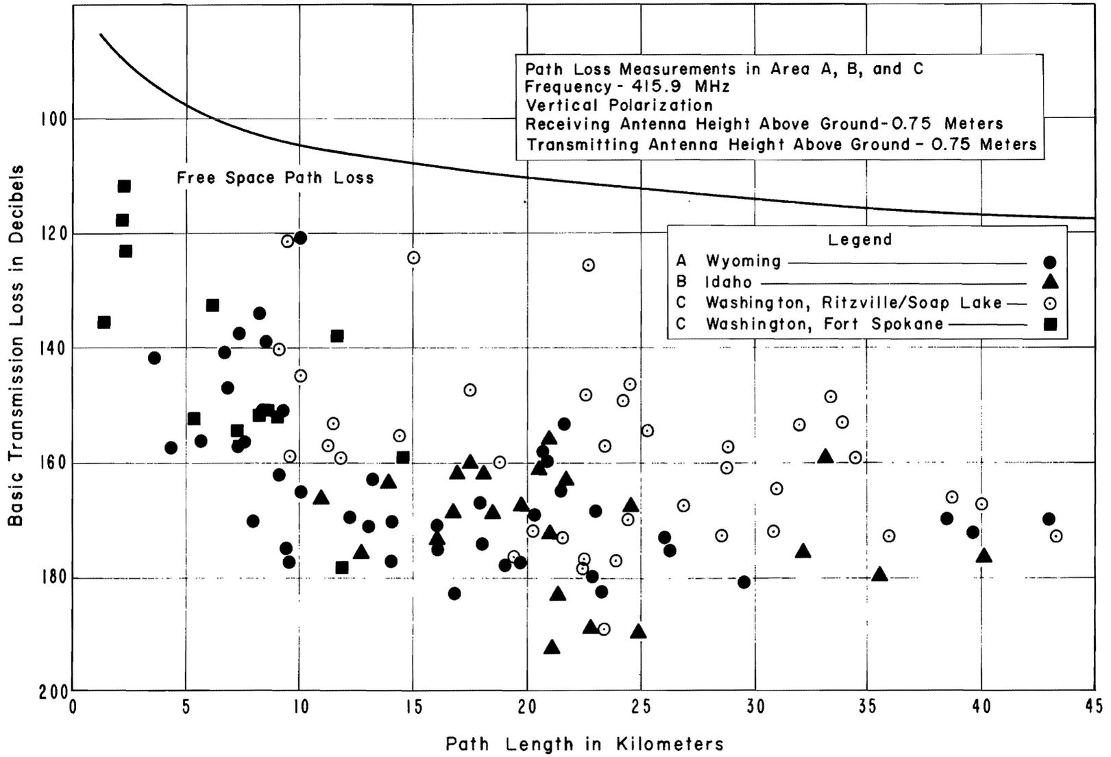
Figure 25. Basic transmission loss for all paths.
