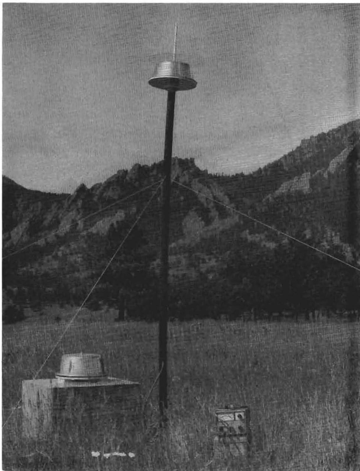
Figure 8. Transmitting antenna at 3.0 m height
