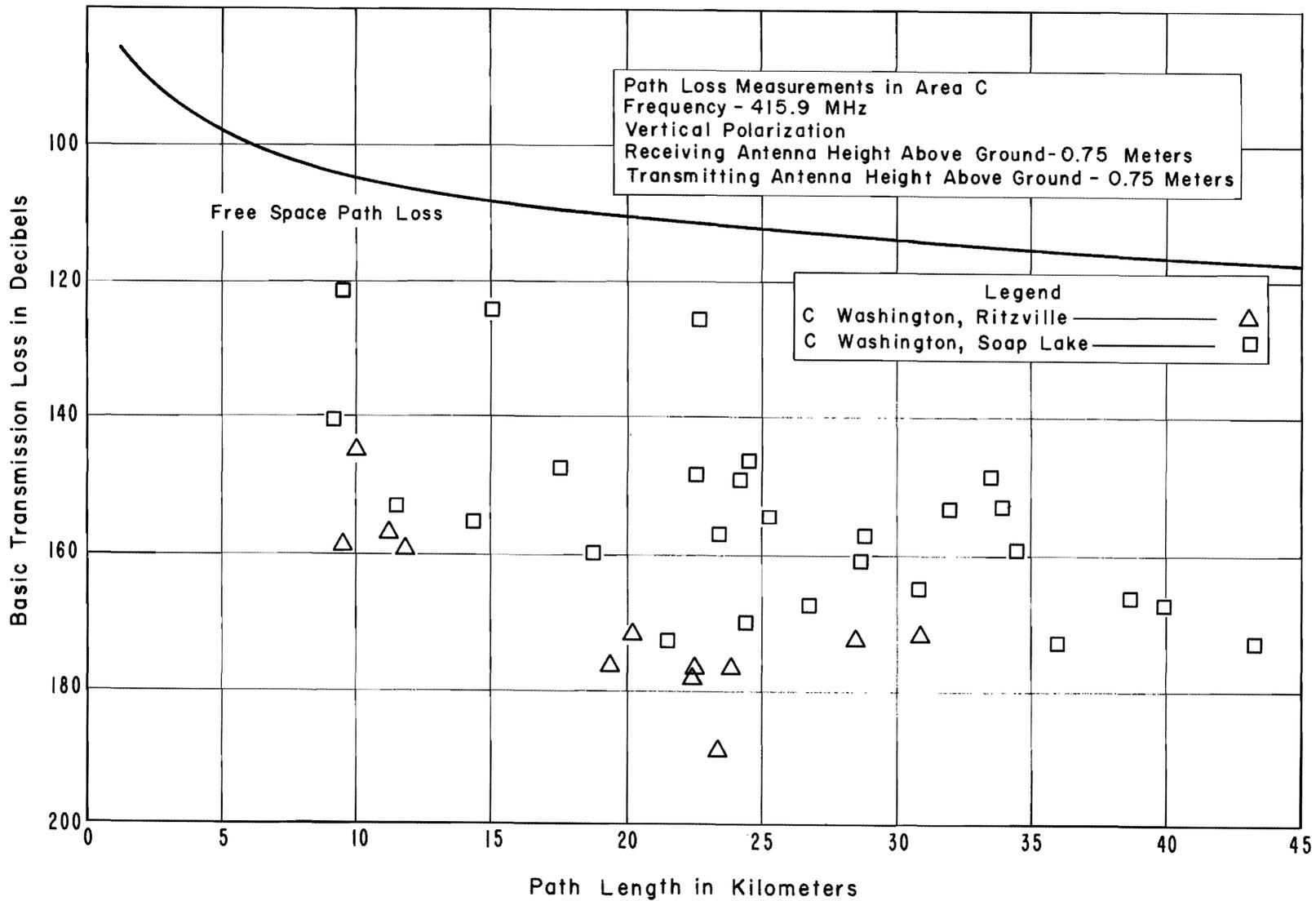
Figure 26. Basic transmission loss Washington intra-area comparison
