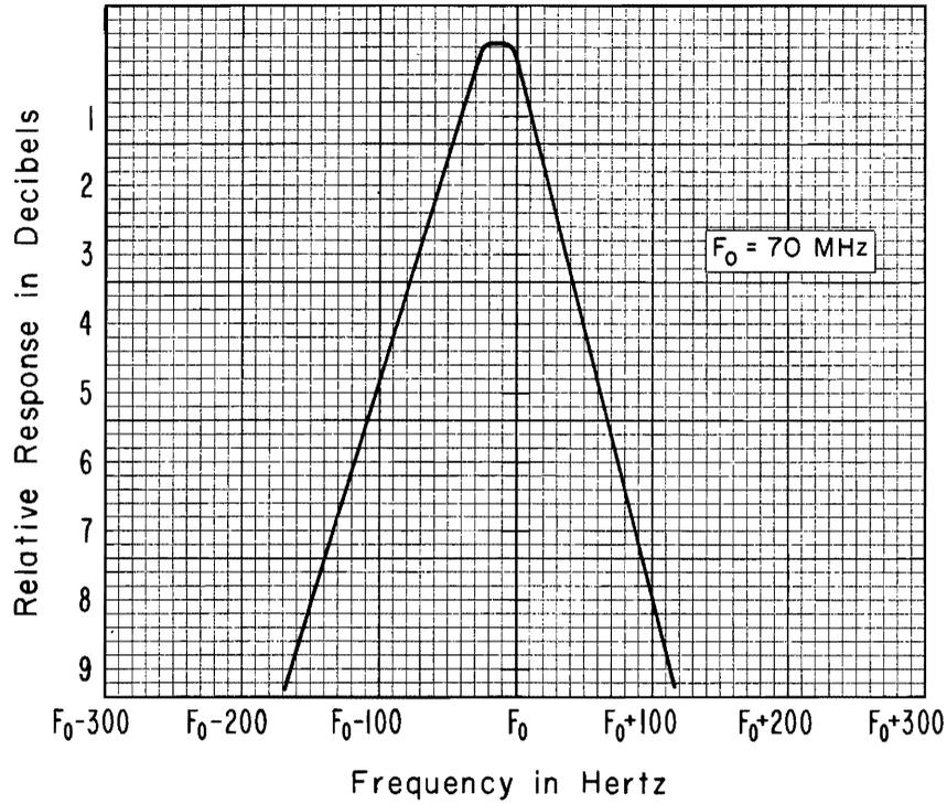
Figure 12. IF filter characteristic
