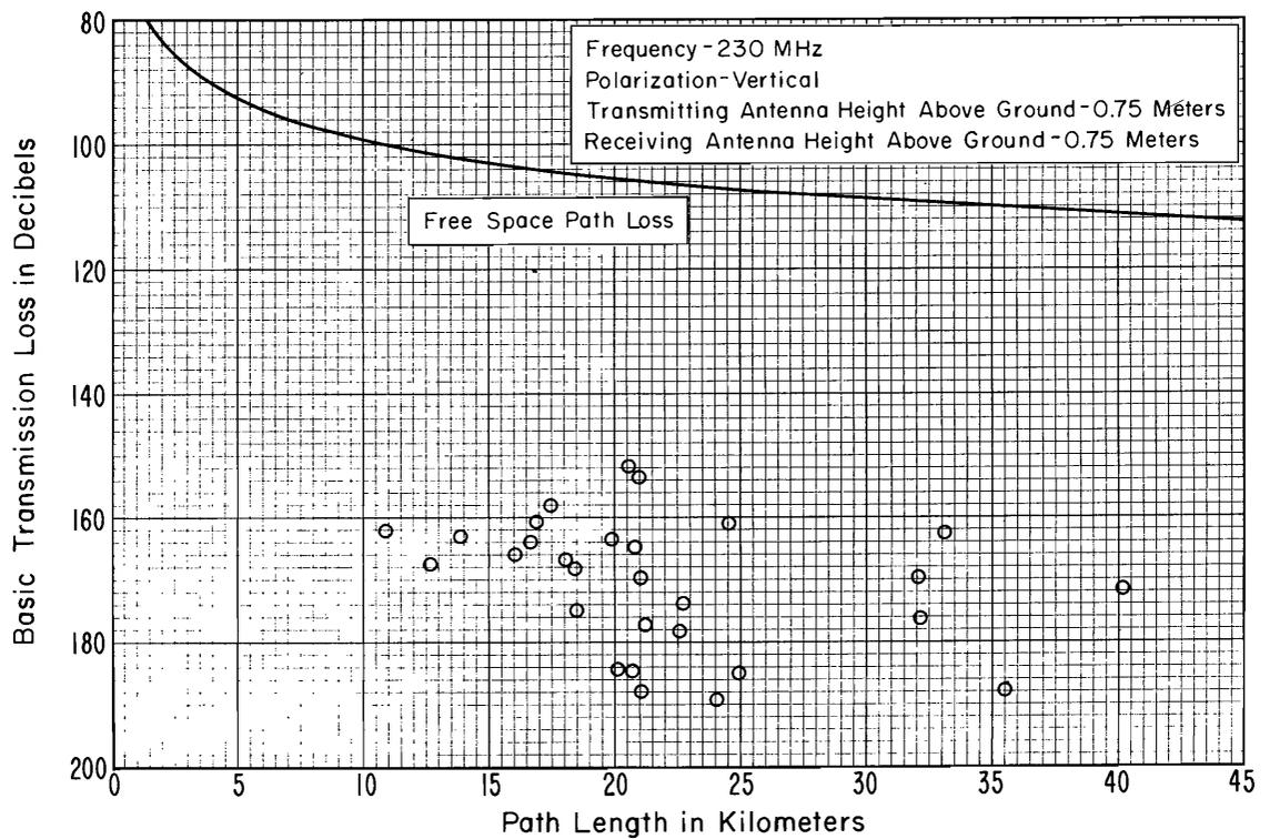
Figure 18. Idaho area radio path loss at 230 MHz
