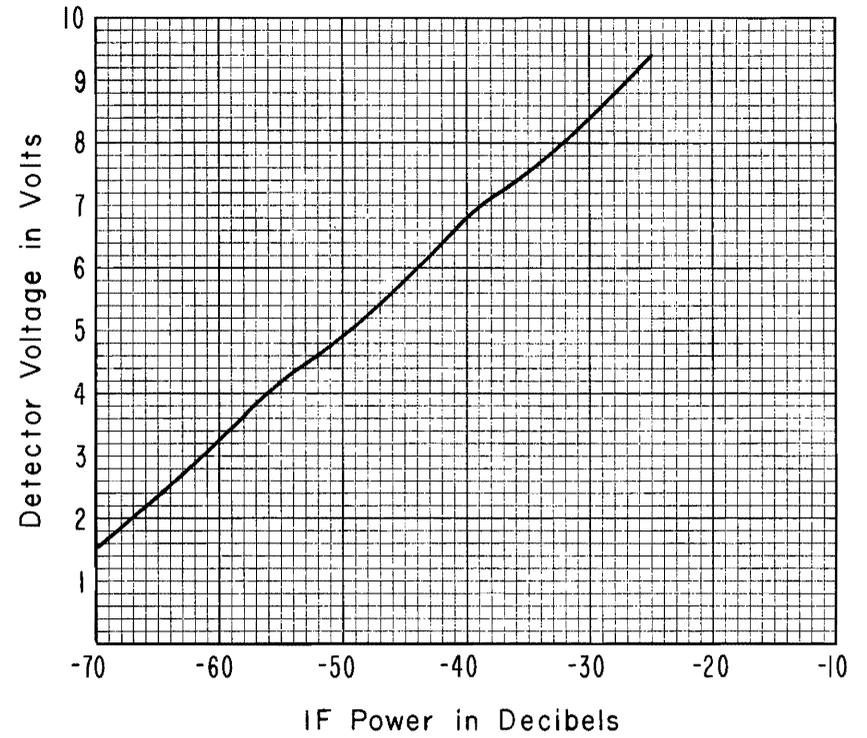
Figure 13. Log linear IF amplifier (70 MHz) dynamic range
