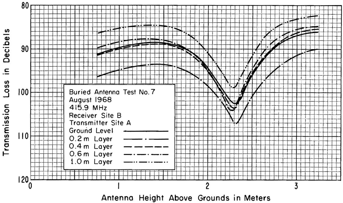
Figure 49. Buried antenna test results for test no. 7.
