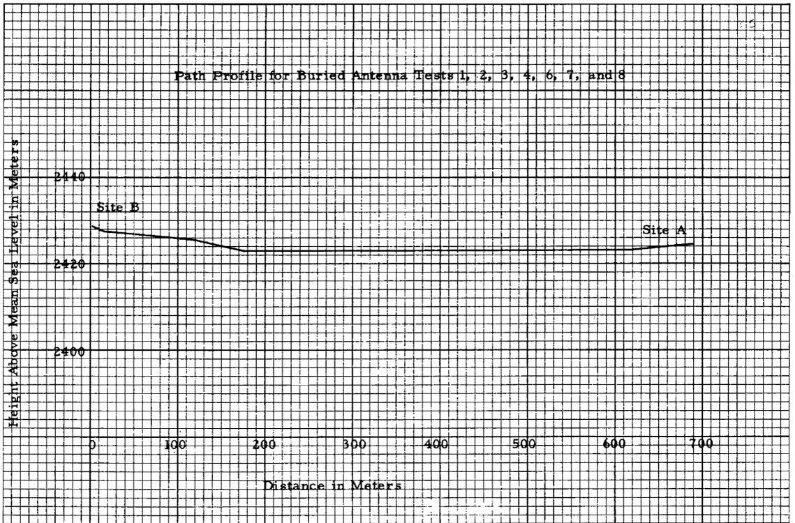
Figure 35. Path profile for buried antenna tests 1, 2, 3, 4, 6, 7, and 8.
