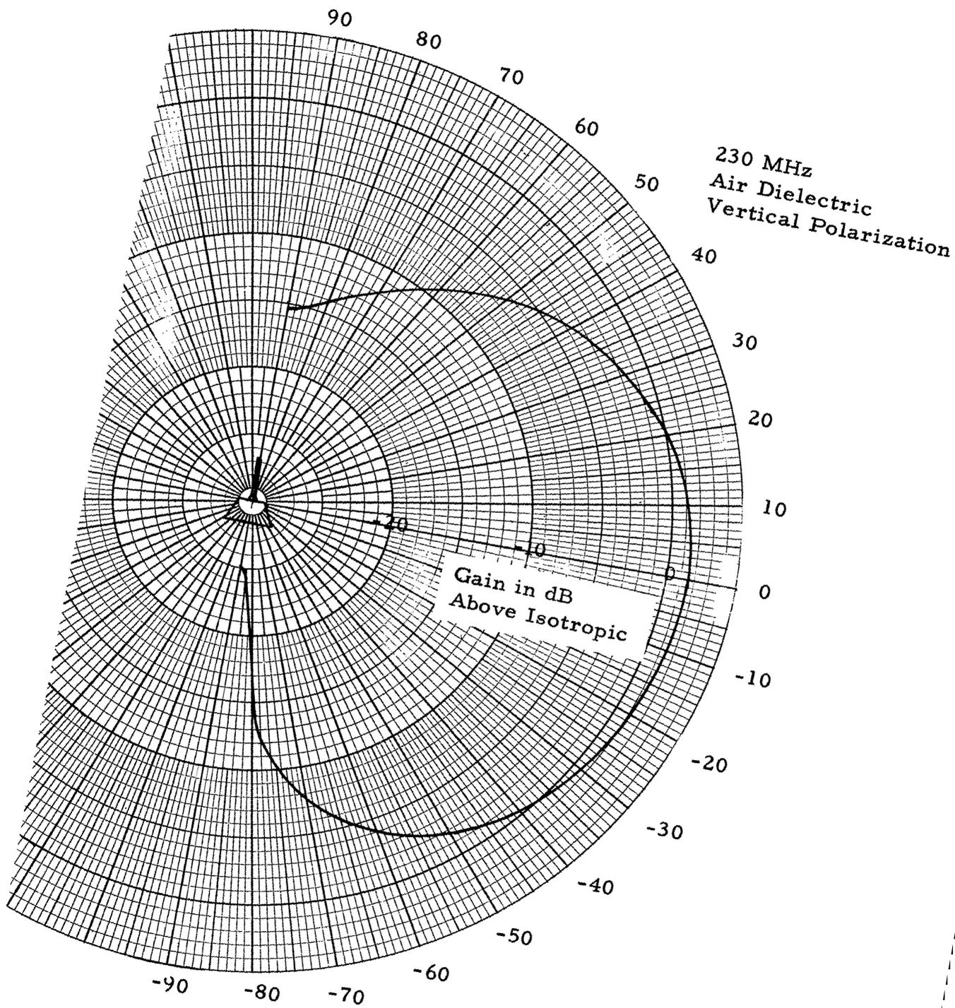
Figure 10. Stub antenna vertical pattern for 230 MHz
