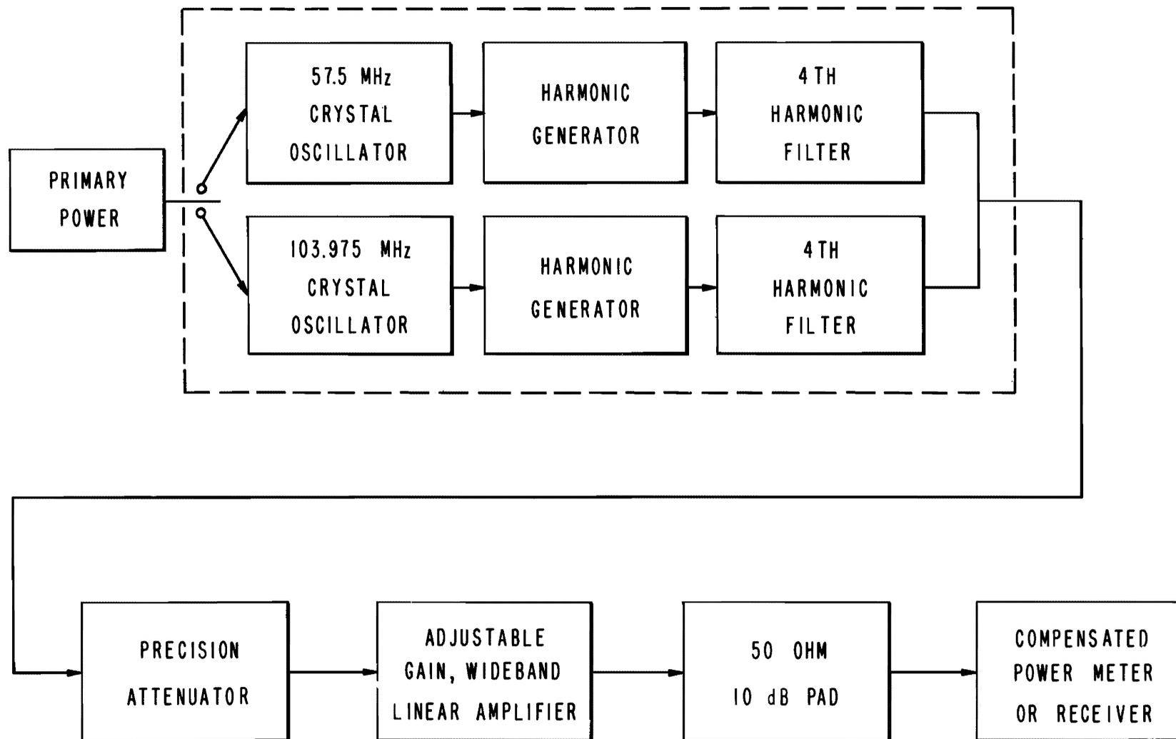
Figure 14. Signal generator block diagram
