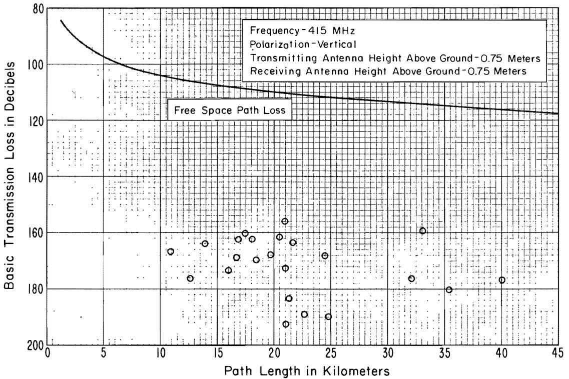
Figure 19. Idaho area radio path loss at 415.9 MHz
