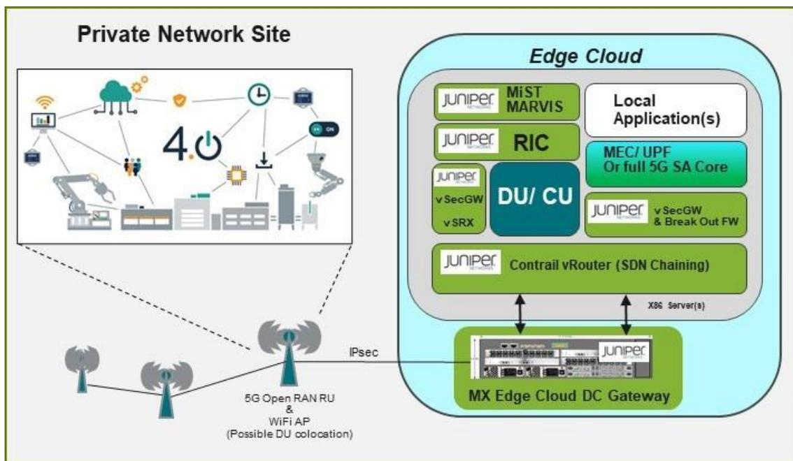
As can be seen from the green building blocks in the diagram, Juniper proposes to integrate 5G SA Core / MEC and ORAN components with routing, switching, security and cloud capabilities to deliver a private network that can be used to assess the benefit of using 5G as the connectivity solution for a variety of applications.
