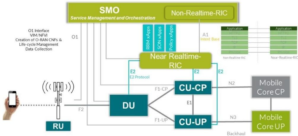
The RIC could host an application that is linked to the other DoD systems and hence can control the RF power and spectrum band being used by the 5G system allowing dynamic sharing.
