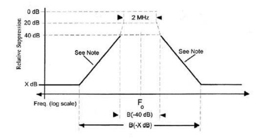
Note: The roll-off slope, S, from the -40 dB to -X dB points is at 40 dB per decade for Criteria E. The -20 dB bandwidth is limited to 2 MHz for Wind Profiler radars operating at 449 MHz. The maximum emission spectrum level between the -40 dB and -X dB points for S dB per decade slope is described by the formula:
