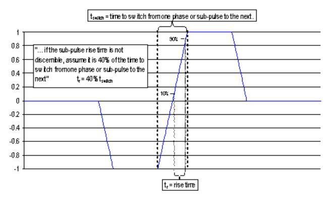
FIGURE 3. Estimation of chip rise time for phase coded pulse signals
