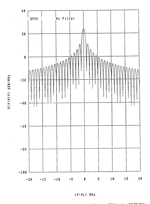
Modulating bit rate = 2.00 mps Power = 250.00 watts 99% band = 18.75 MHz Figure 2-5. Power spectral density QPSK with NRZ modulation.
