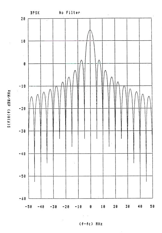
Modulating bit rate = 5.00 mps Power = 150.00 watts 99% band = 78.13 MHz
