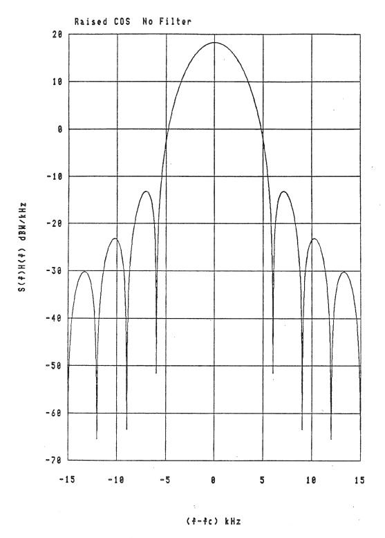
Modulating bit rate = 3.00 kps Power = 300.00 watts 99% band = 8.50 kHz
