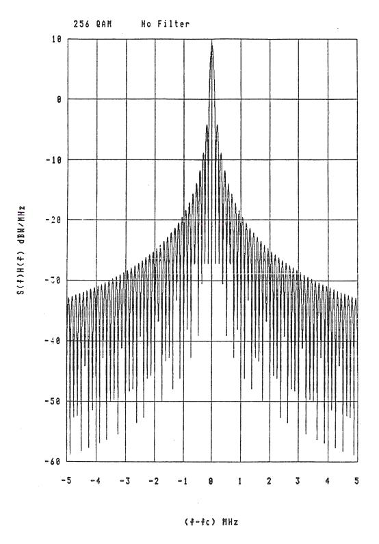
Modulating bit rate = 1.00 mps Power = 1.00 watts 99% band = 2.34 MHz
