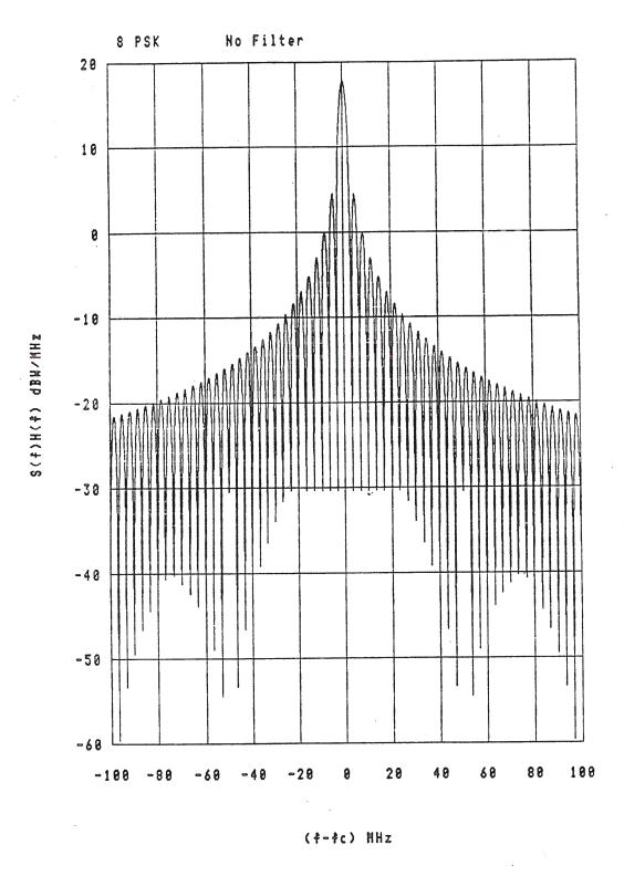
Modulating bit rate = 10.00 mps Power = 200.00 watts 99% band = 62.50 MHz
