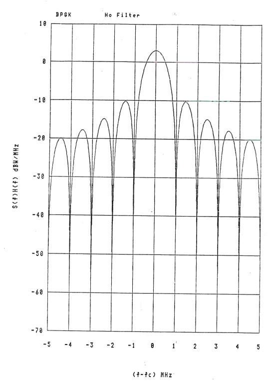
Modulating bit rate = 1.00 mps Power = 2.00 watts 99% band = 15.63 MHz
