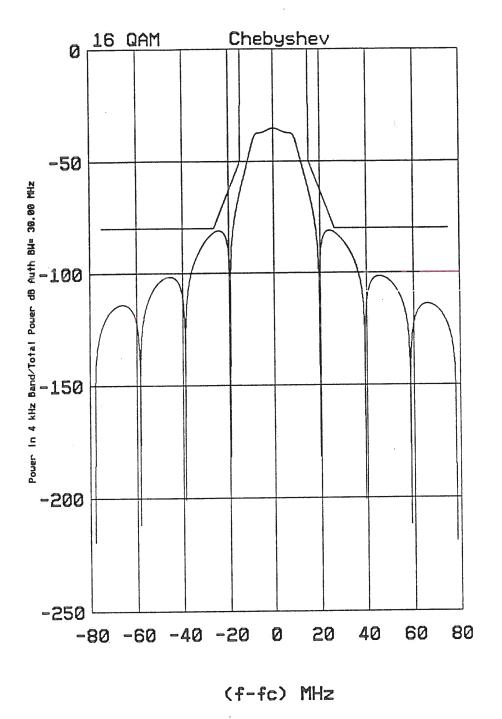
Modulating bit rate = 78.0 mps Power = 1.00 watts 99% band = 21.42 MHz
