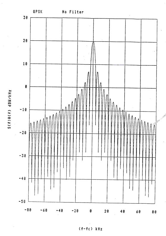
Modulating bit rate = 8.00 kps Power = 400.00 watts 99% band = 75.00 kHz Figure 2-6. Power spectral density QPSK with NRZ modulation.
