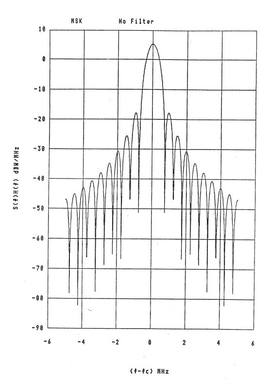
Modulating bit rate = 1.00 mps Power = 2.00 watts 99% band = 1.17 MHz
