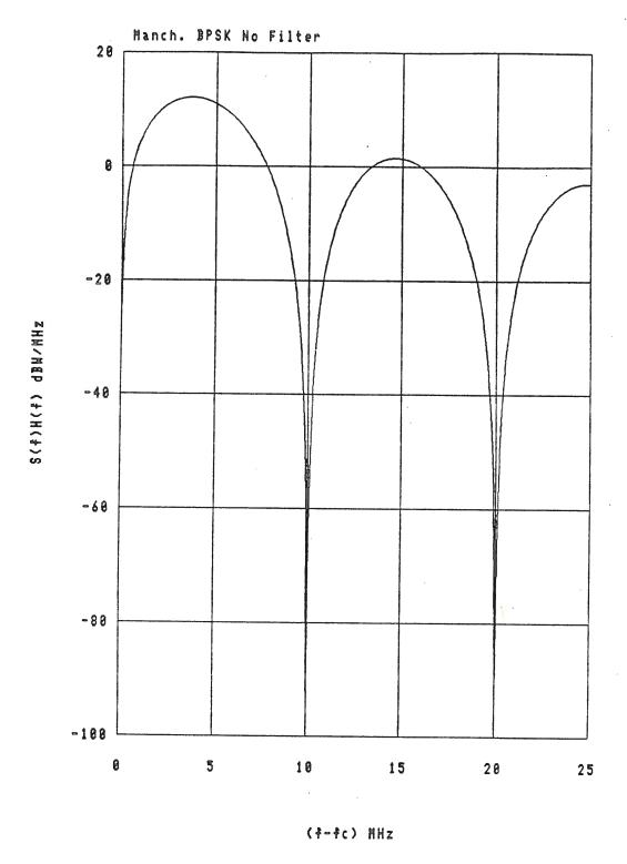
Modulating bit rate = 5.00 mps Power = 150.00 watts 99% band = 140.63 MHz
