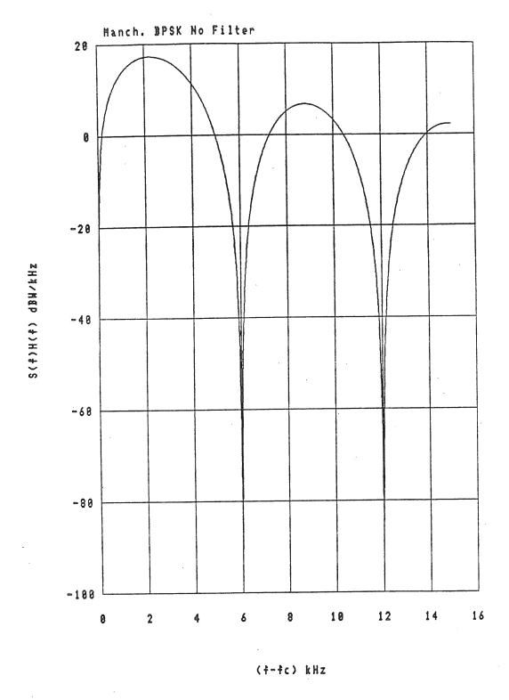
Modulating bit rate = 3.00 kps Power = 300.00 watts 99% band = 84.38 kHz
