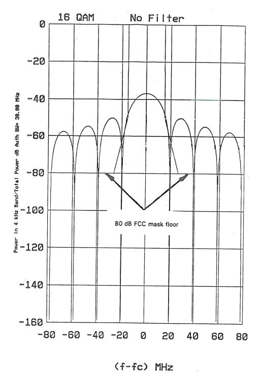
Modulating bit rate = 78.0 mps Power = 1.00 watts 99% band = 365.63 MHz FCC Mask for 6 GHz band and 30 MHz authorized bandwidth.
