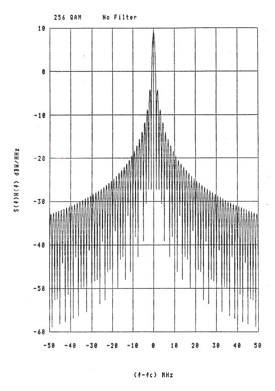
Modulating bit rate = 10.00 mps Power = 10.00 watts 99% band = 23.44 MHz
