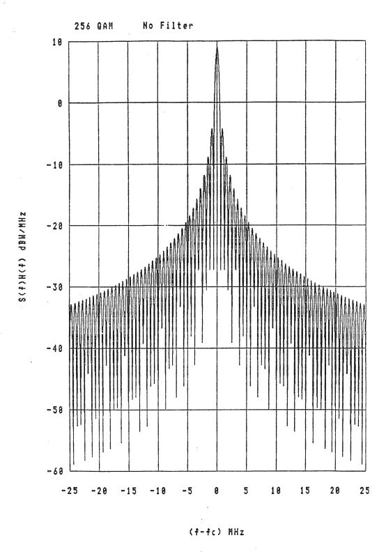
Modulating bit rate = 5.00 mps Power = 5.00 watts 99% band = 11.72 MHz
