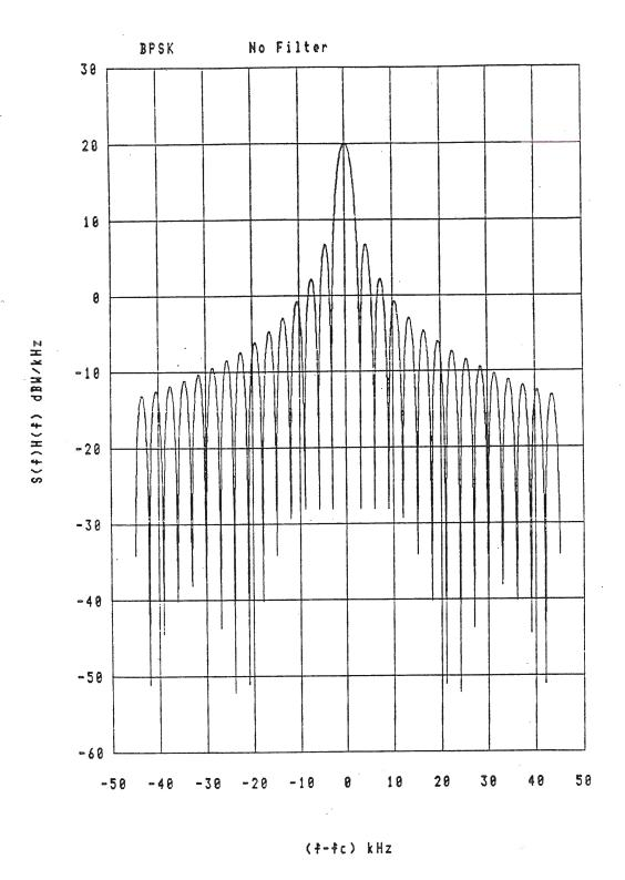
Modulating bit rate = 3.00 kps Power = 300.00 watts 99% band = 46.88 kHz Figure 2-2. Power spectral density BPSK with NRZ modulation.
