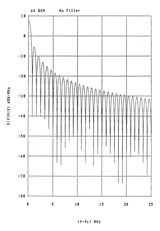
Modulating bit rate = 5.00 mps Power = 5.00 watts 99% band = 15.63 MHz
