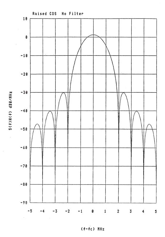
Modulating bit rate = 1.00 mps Power = 2.00 watts 99% band = 2.83 MHz Figure 2-23. Power spectral density BPSK with raised cosine modulation.
