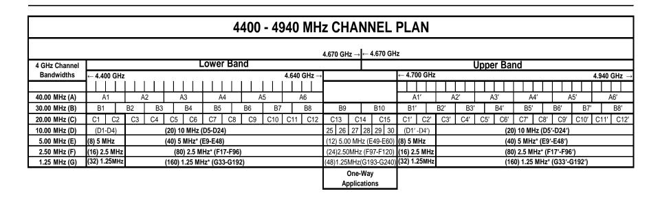
NOTE: Paired channels will be implemented for fixed service assignments using A1 with A1', A2 with A2', etc.
