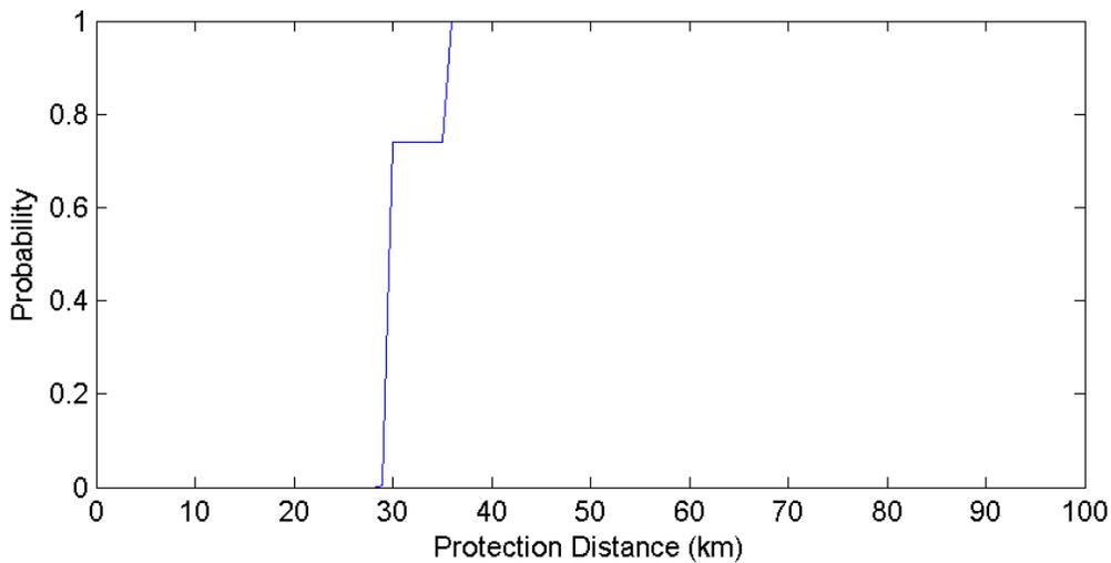
**Figure 74. Elmendorf AFB Alaska POES Protection Distances – 10 MHz Channel (500 Iterations)**
