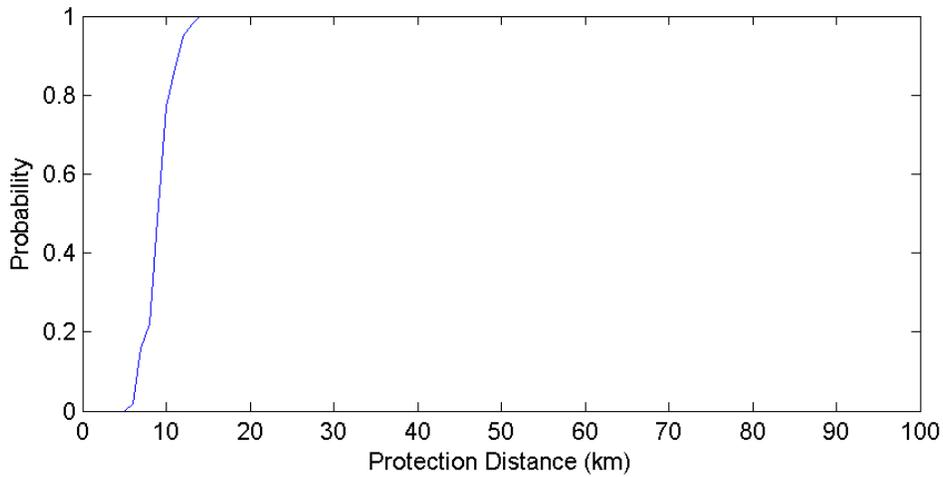
**Figure 51. Vicksburg Mississippi GOES Protection Distances – 15 MHz Channel (500 Iterations)**
