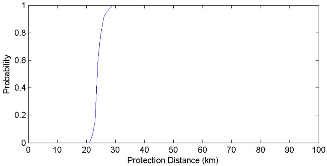
**Figure 94. Boise Idaho GOES Protection Distances – 5 MHz Channel (500 Iterations)**
