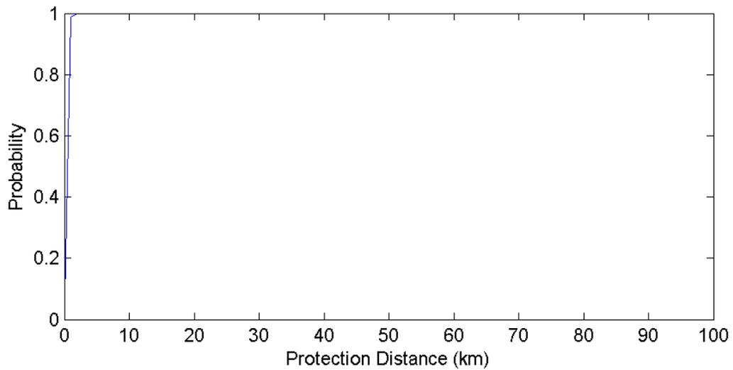
**Figure 22. Miami Florida GOES Protection Distances – 5 MHz Channel (500 Iterations)**
