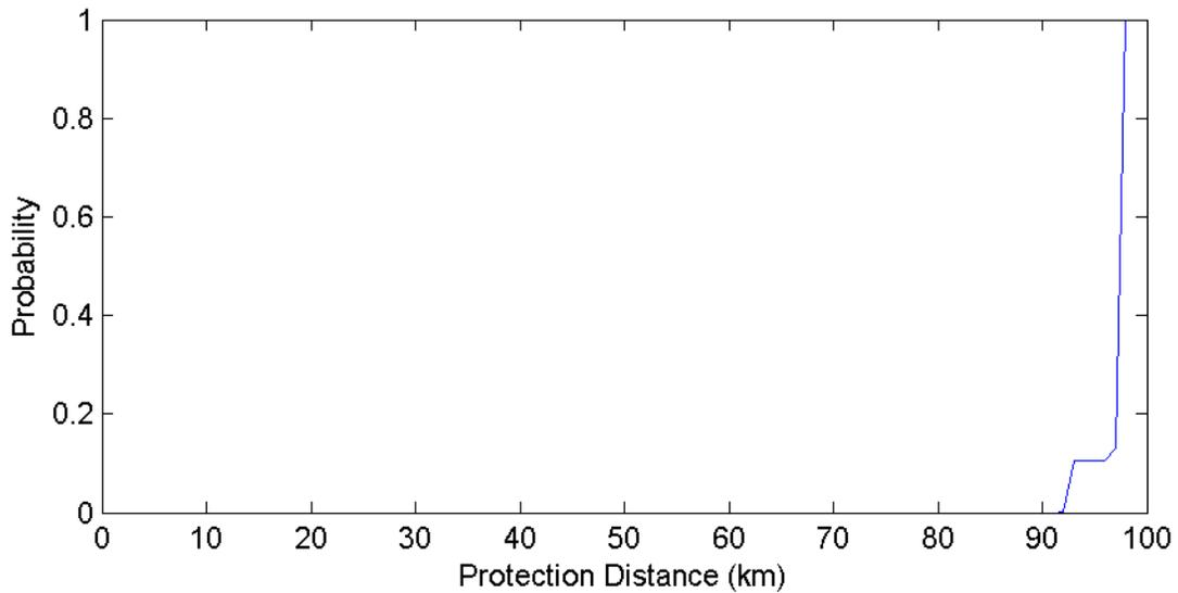
**Figure 72. Elmendorf AFB Alaska POES Protection Distances – 15 MHz Channel (500 Iterations)**
