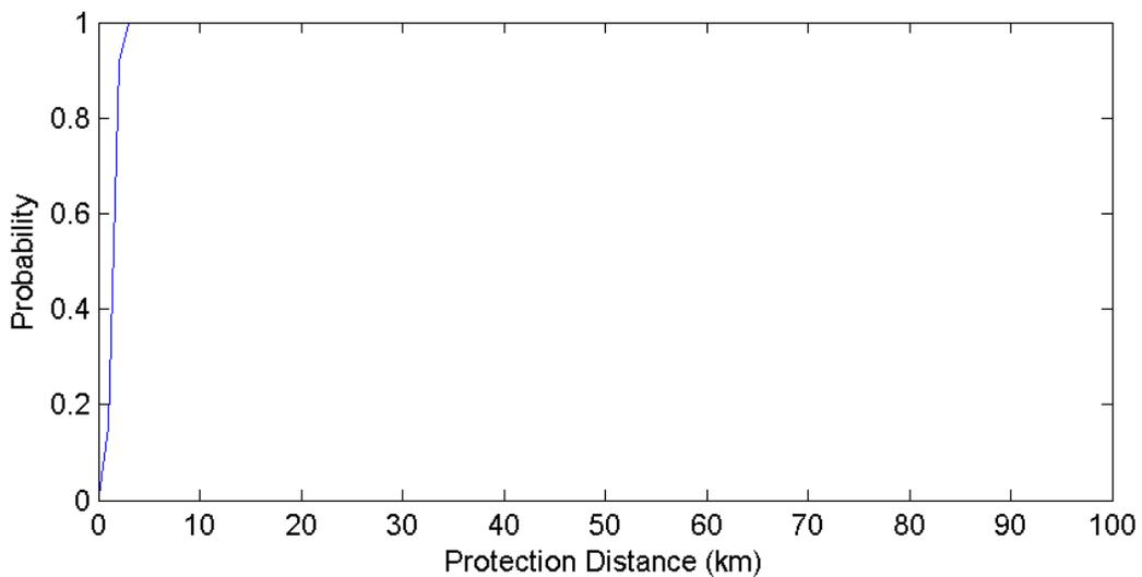
**Figure 117. Greenbelt Maryland GOES Protection Distances – 10 MHz Channel (500 Iterations)**
