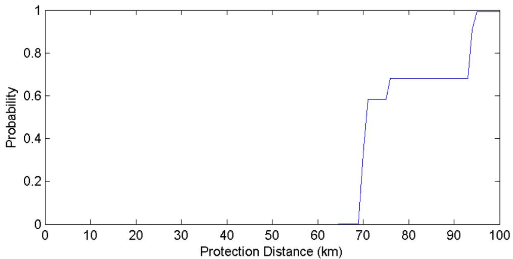
**Figure 86. Yuma Arizona POES Protection Distances – 10 MHz Channel (500 Iterations)**
