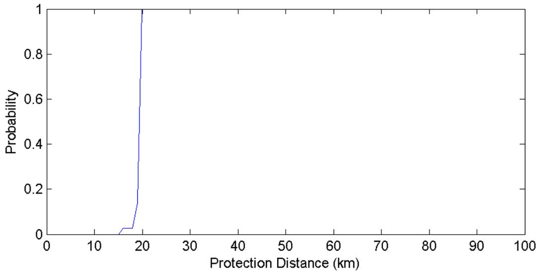
**Figure 8. Fairbanks Alaska POES Protection Distances – 10 MHz Channel (500 Iterations)**
