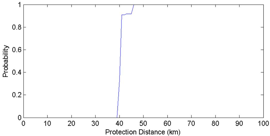
**Figure 17. Miami Florida POES Protection Distances – 10 MHz Channel (500 Iterations)**
