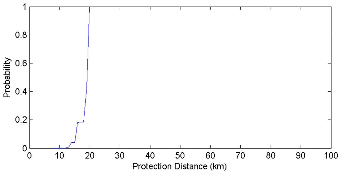
**Figure 7. Fairbanks Alaska POES Protection Distances – 5 MHz Channel (500 Iterations)**
