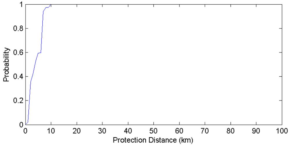
**Figure 140. San Juan Puerto Rico GOES Protection Distances – 5 MHz Channel (500 Iterations)**
