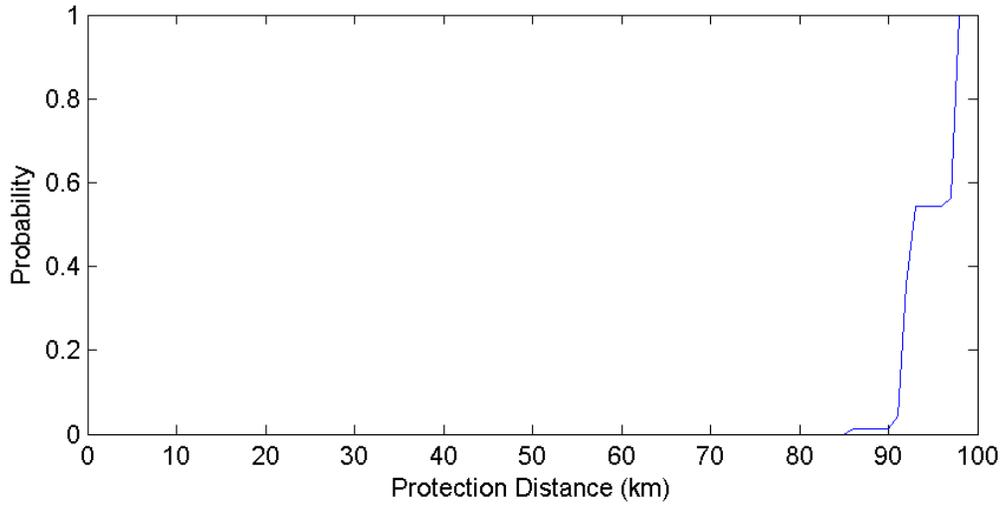
**Figure 70. Elmendorf AFB Alaska POES Protection Distances – 5 MHz Channel (500 Iterations)**
