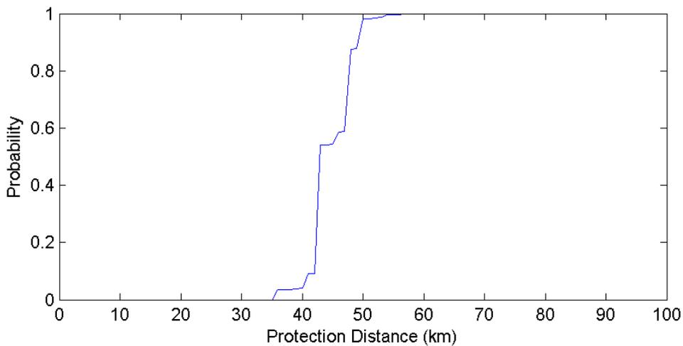
**Figure 80. Stennis Space Center Mississippi POES Protection Distances – 10 MHz Channel (500 Iterations)**
