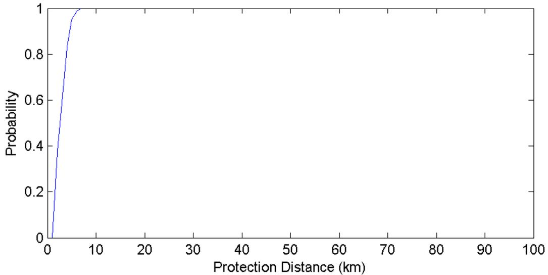
**Figure 90. Anchorage Alaska GOES Protection Distances – 15 MHz Channel (500 Iterations)**
