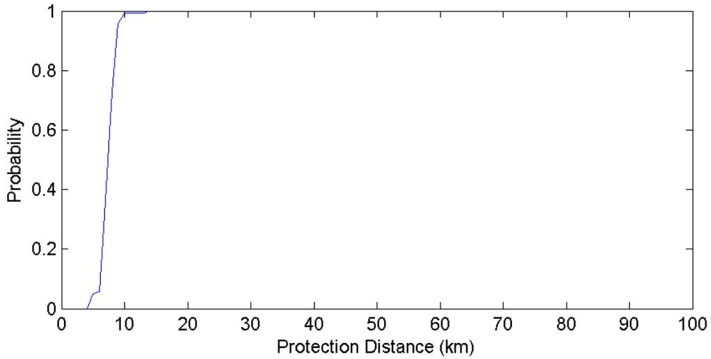
**Figure 37. Rock Island Illinois GOES Protection Distances – 5 MHz Channel (500 Iterations)**
