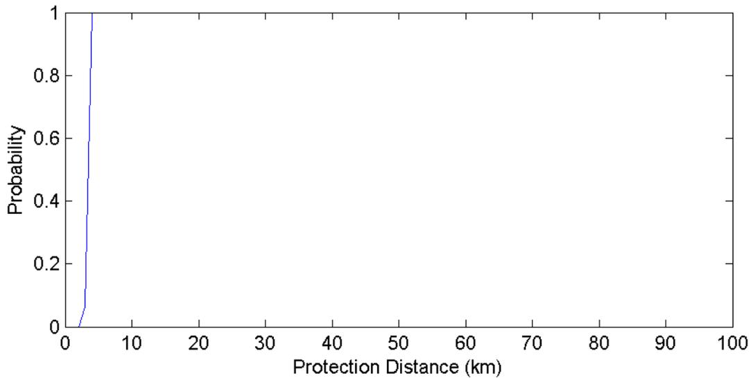
**Figure 115. Fairmont West Virginia GOES Protection Distances – 15 MHz Channel (500 Iterations)**
