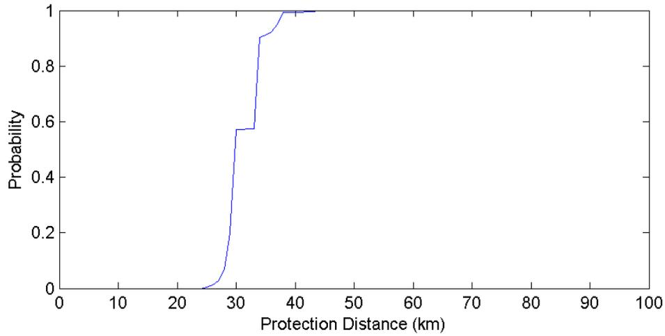
**Figure 137. Guaynabo Puerto Rico GOES Protection Distances – 5 MHz Channel (500 Iterations)**
