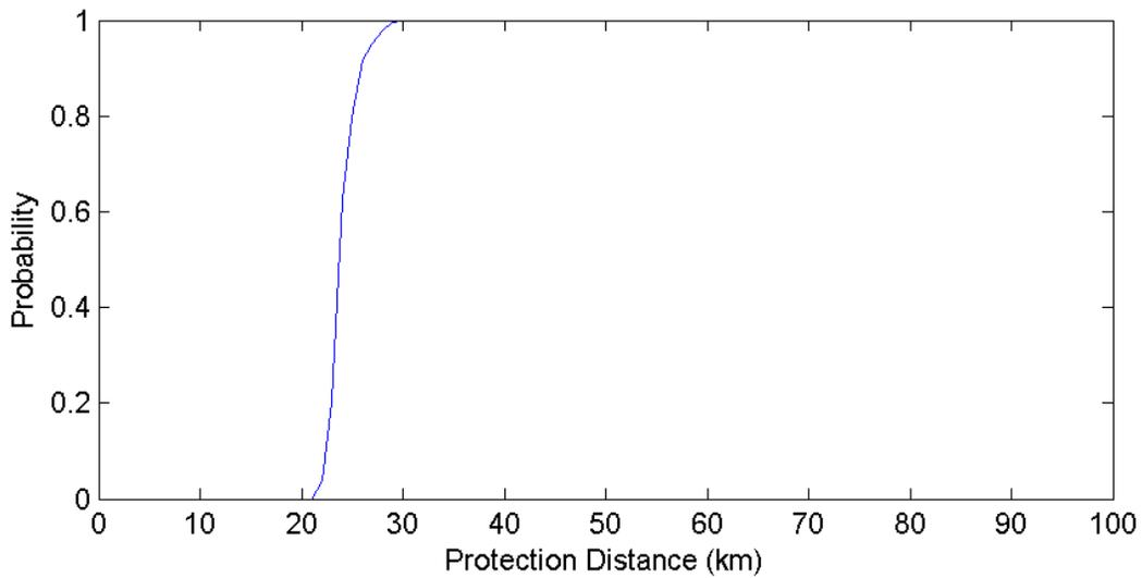
**Figure 95. Boise Idaho GOES Protection Distances – 10 MHz Channel (500 Iterations)**
