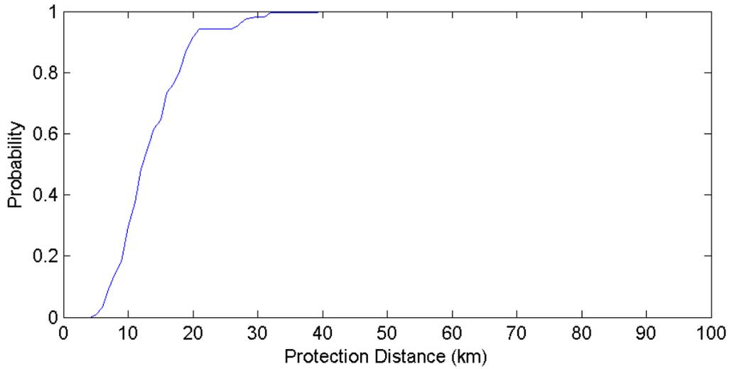
**Figure 119. Knoxville Tennessee GOES Protection Distances – 5 MHz Channel (500 Iterations)**
