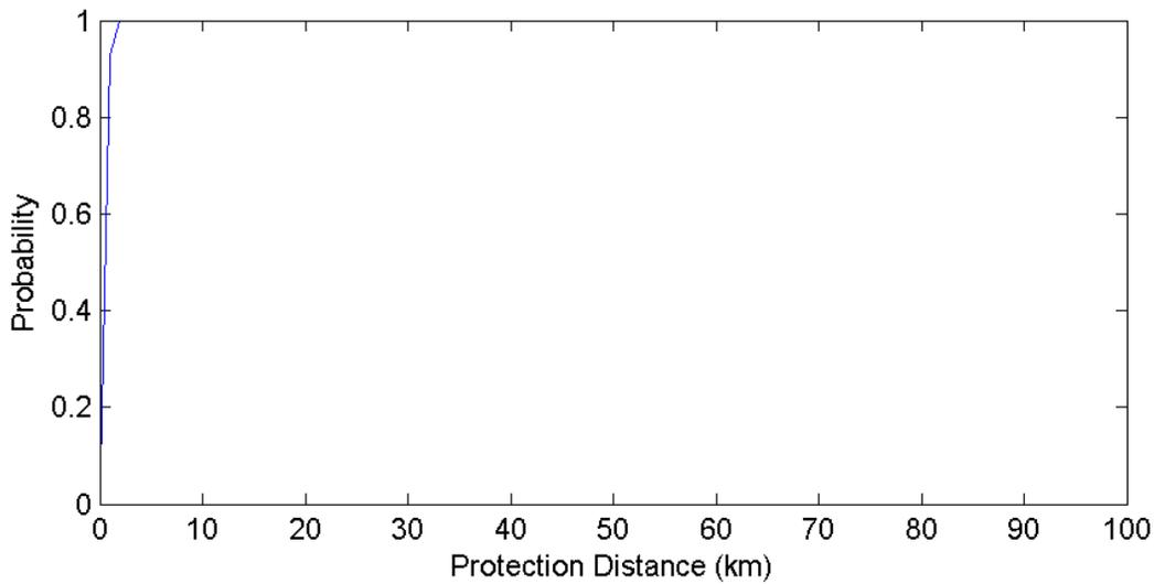
**Figure 101. Boulder Colorado GOES Protection Distances – 10 MHz Channel (500 Iterations)**
