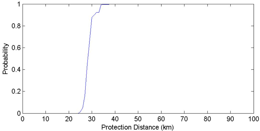
**Figure 112. Kansas City Missouri GOES Protection Distances – 15 MHz Channel (500 Iterations)**
