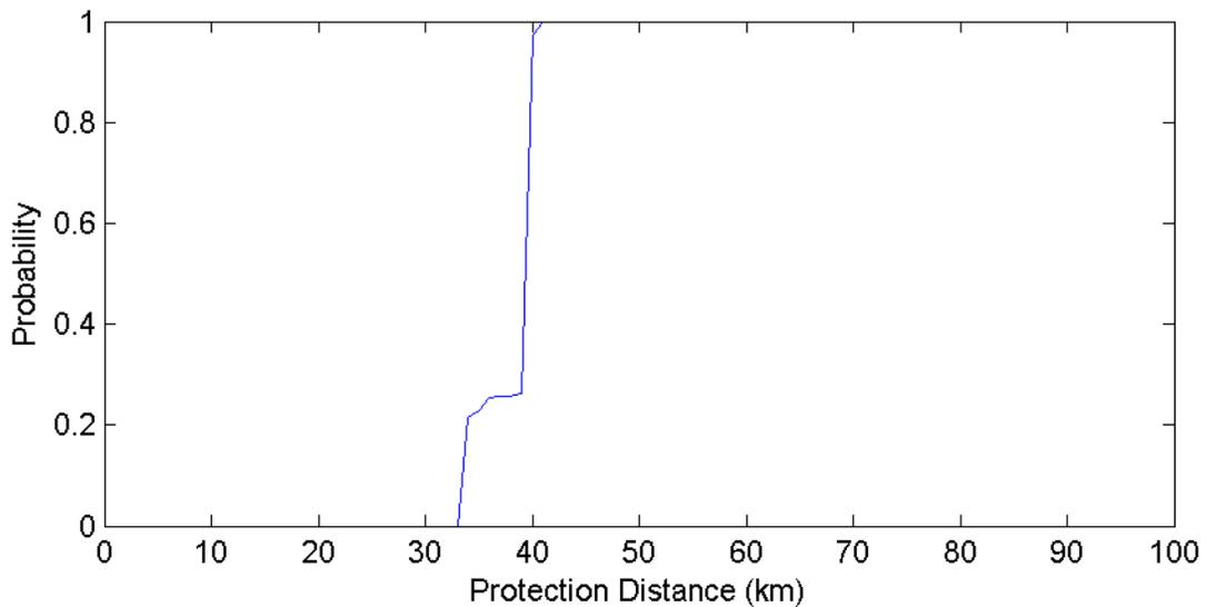
**Figure 16. Miami Florida POES Protection Distances – 5 MHz Channel (500 Iterations)**
