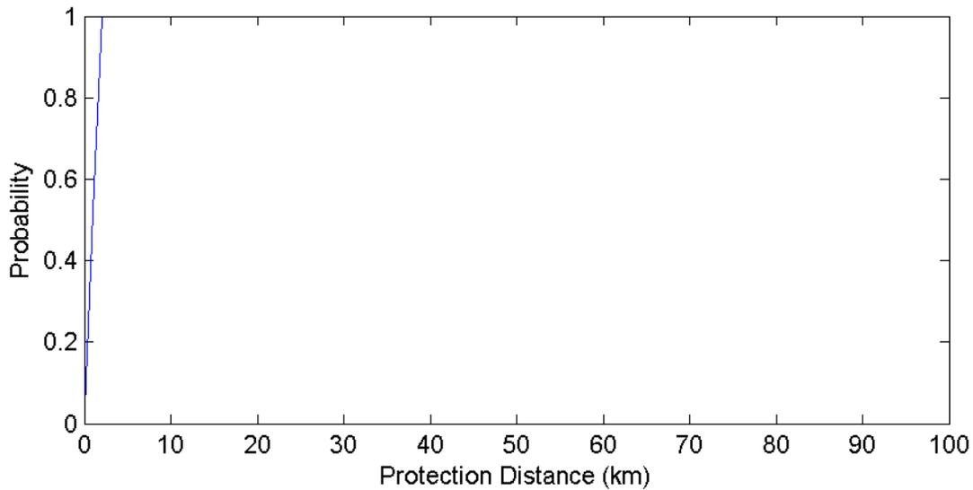
**Figure 133. Sioux Falls South Dakota GOES Protection Distances – 15 MHz Channel (500 Iterations)**
