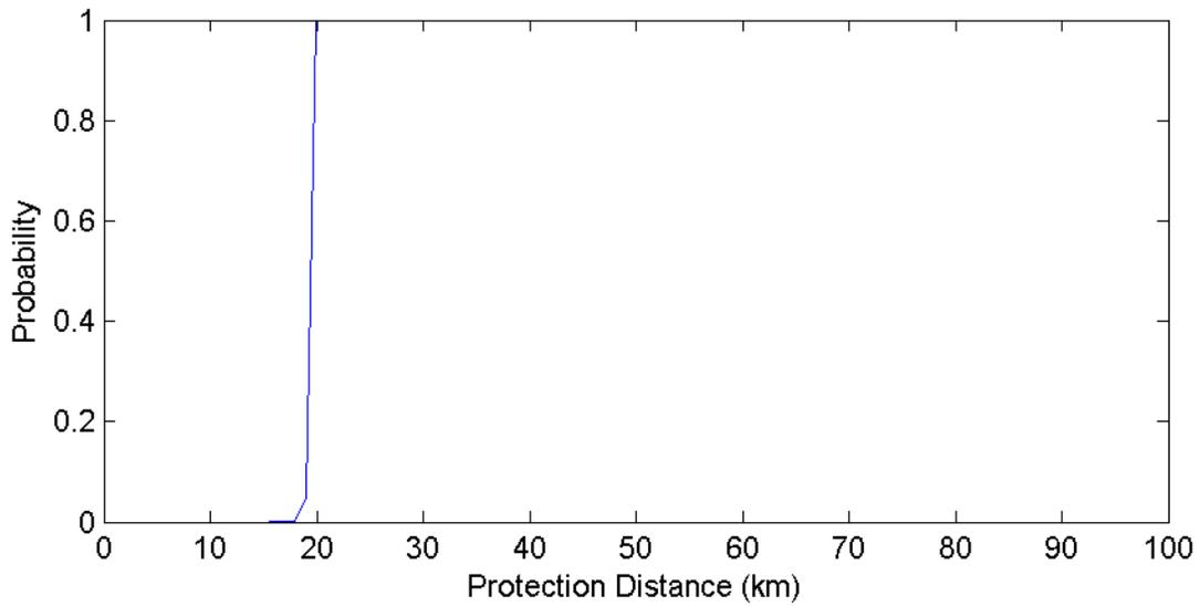
**Figure 9. Fairbanks Alaska POES Protection Distances – 15 MHz Channel (500 Iterations)**
