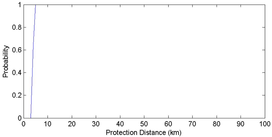
**Figure 6. Wallops Island Virginia GOES Protection Distances – 15 MHz Channel (500 Iterations)**
