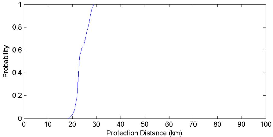
**Figure 98. Boise Idaho GOES Protection Distances – 10 MHz Channel (500 Iterations)**
