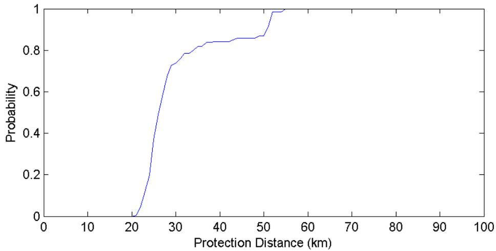
**Figure 66. Sacramento California GOES Protection Distances – 15 MHz Channel (500 Iterations)**
