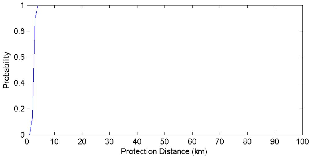
**Figure 118. Greenbelt Maryland GOES Protection Distances – 15 MHz Channel (500 Iterations)**
