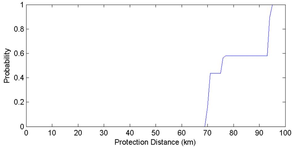
**Figure 87. Yuma Arizona POES Protection Distances – 15 MHz Channel (500 Iterations)**
