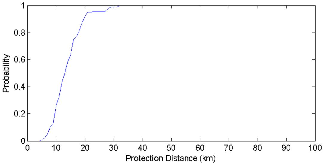
**Figure 121. Knoxville Tennessee GOES Protection Distances – 15 MHz Channel (500 Iterations)**
