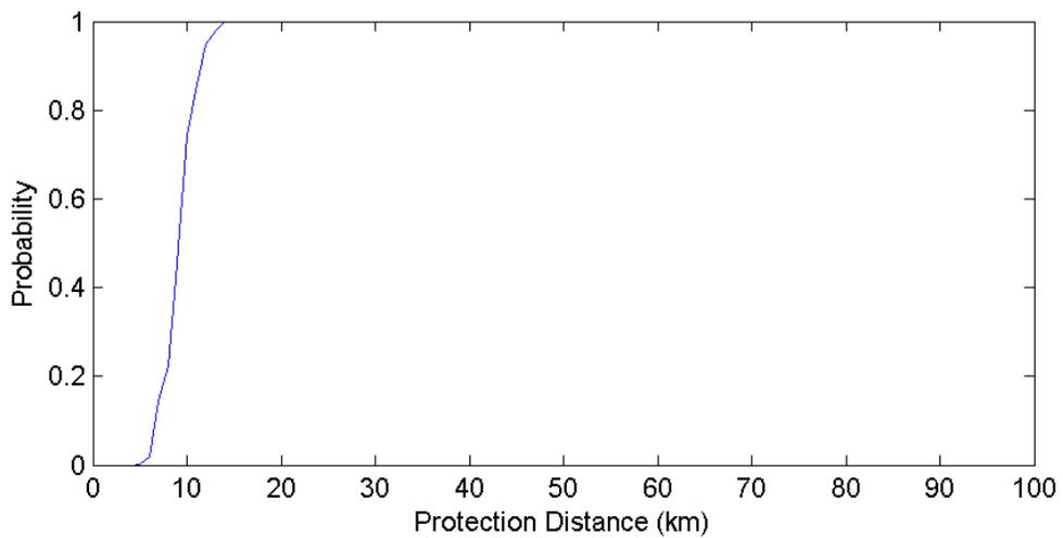
**Figure 50. Vicksburg Mississippi GOES Protection Distances – 10 MHz Channel (500 Iterations)**
