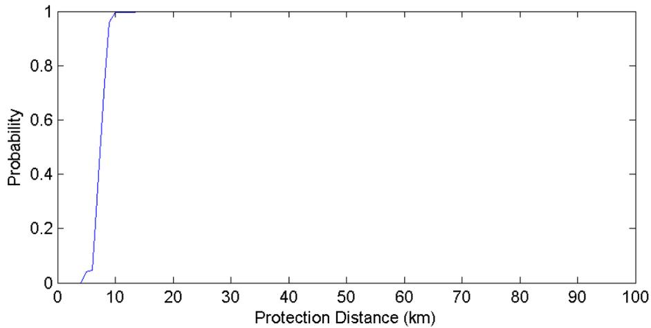
**Figure 39. Rock Island Illinois GOES Protection Distances – 15 MHz Channel (500 Iterations)**
