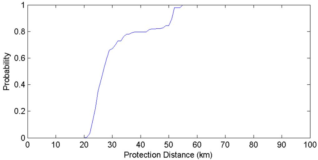
**Figure 64. Sacramento California GOES Protection Distances – 5 MHz Channel (500 Iterations)**
