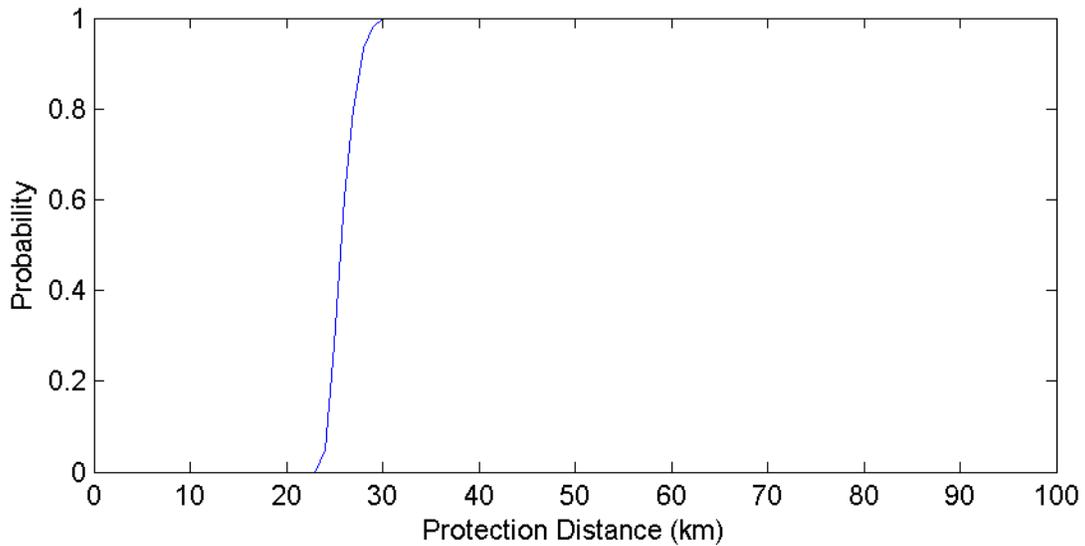
**Figure 130. Sioux Falls South Dakota GOES Protection Distances – 15 MHz Channel (500 Iterations)**
