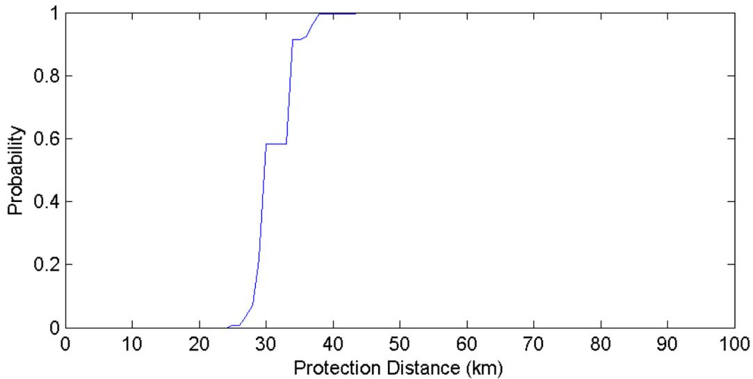
**Figure 139. Guaynabo Puerto Rico GOES Protection Distances – 15 MHz Channel (500 Iterations)**
