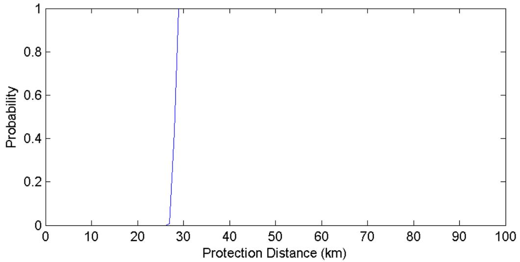
**Figure 21. Miami Florida POES Protection Distances – 15 MHz Channel (500 Iterations)**
