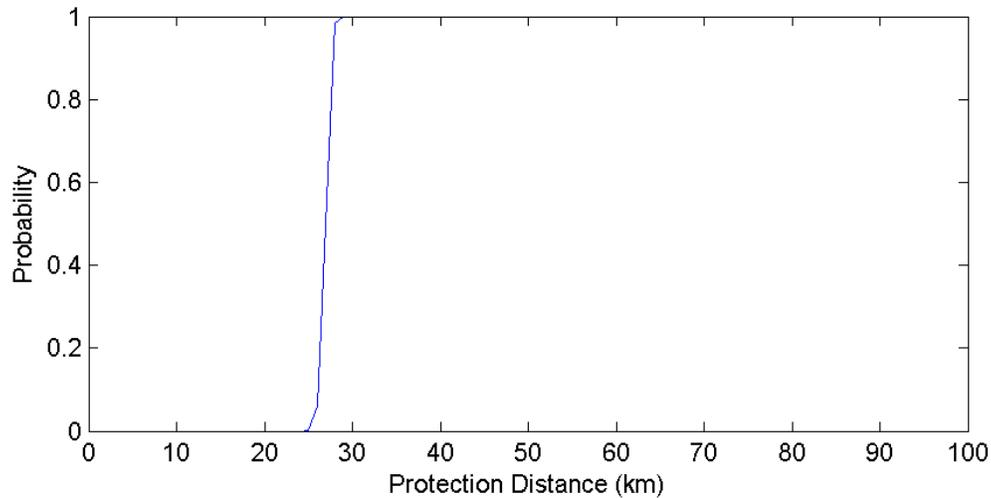
**Figure 1. Wallops Island Virginia POES Protection Distances – 5 MHz Channel (500 Iterations)**
