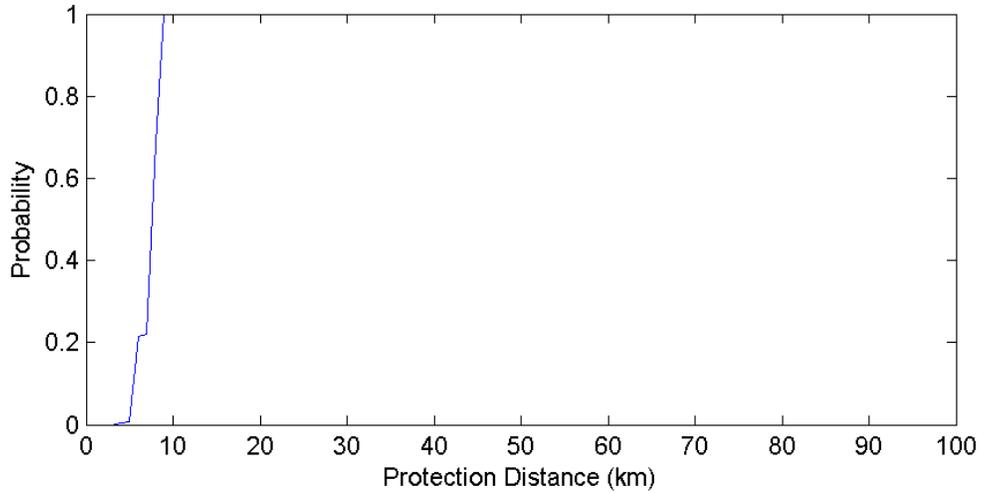
**Figure 155. Anderson AFB Guam POES Protection Distances – 5 MHz Channel (500 Iterations)**
