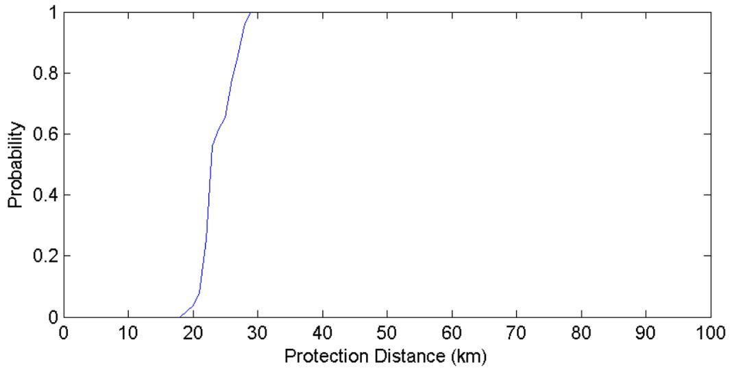
**Figure 97. Boise Idaho GOES Protection Distances – 5 MHz Channel (500 Iterations)**
