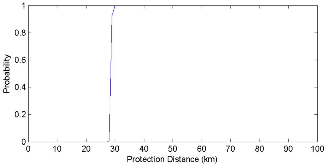
**Figure 2. Wallops Island Virginia POES Protection Distances – 10 MHz Channel (500 Iterations)**
