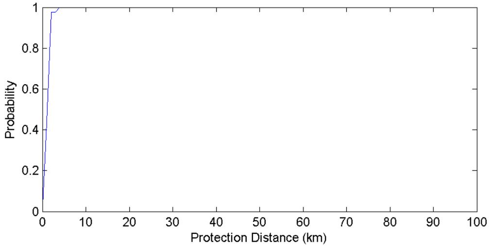
**Figure 152. Barrigada Guam GOES Protection Distances – 5 MHz Channel (500 Iterations)**
