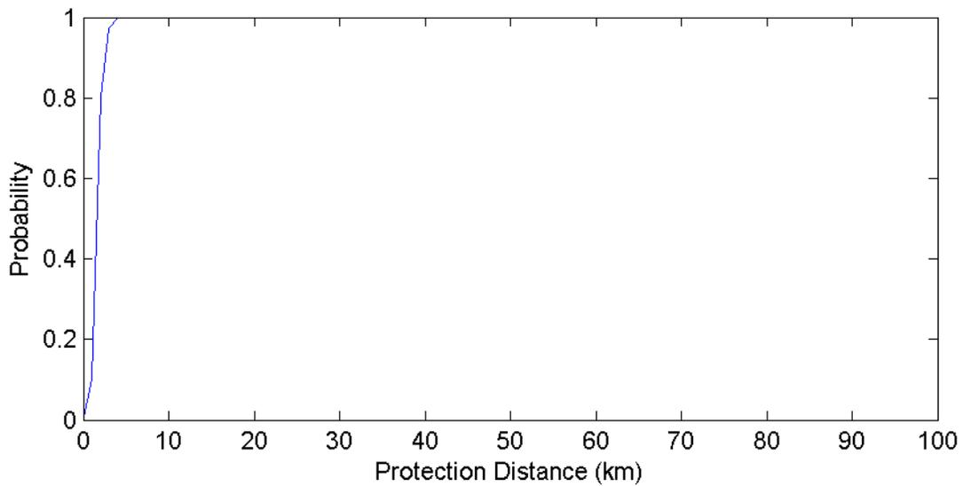
**Figure 4. Wallops Island Virginia GOES Protection Distances – 5 MHz Channel (500 Iterations)**
