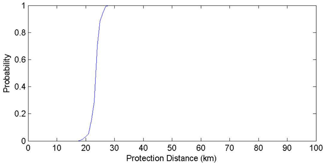
**Figure 127. Sioux Falls South Dakota GOES Protection Distances – 15 MHz Channel (500 Iterations)**
