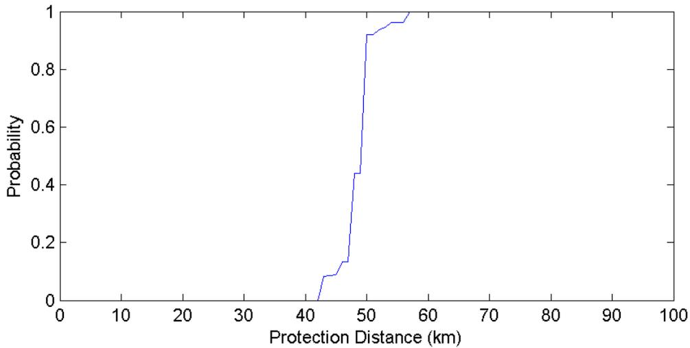
**Figure 81. Stennis Space Center Mississippi POES Protection Distances – 15 MHz Channel (500 Iterations)**
