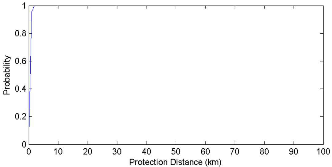
**Figure 23. Miami Florida GOES Protection Distances – 10 MHz Channel (500 Iterations)**
