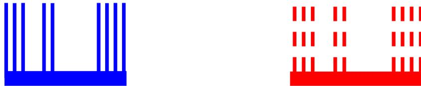
Figure 1, Organized FDMA Band with RX / TX Separation
