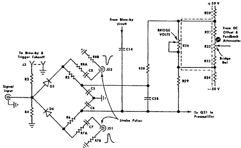
Fig 2.4.2.1 Sampling bridge circuit and Bridge Volts and Bridge Bal circuits. From *Instruction Manual, Type S-2 Sampling Head*, Tektronix, Inc., 1968.
