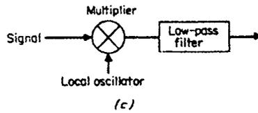
Fig. 14-86. AM detectors: (a) AM envelope detector; (b) peak detector; (c) product detector.
