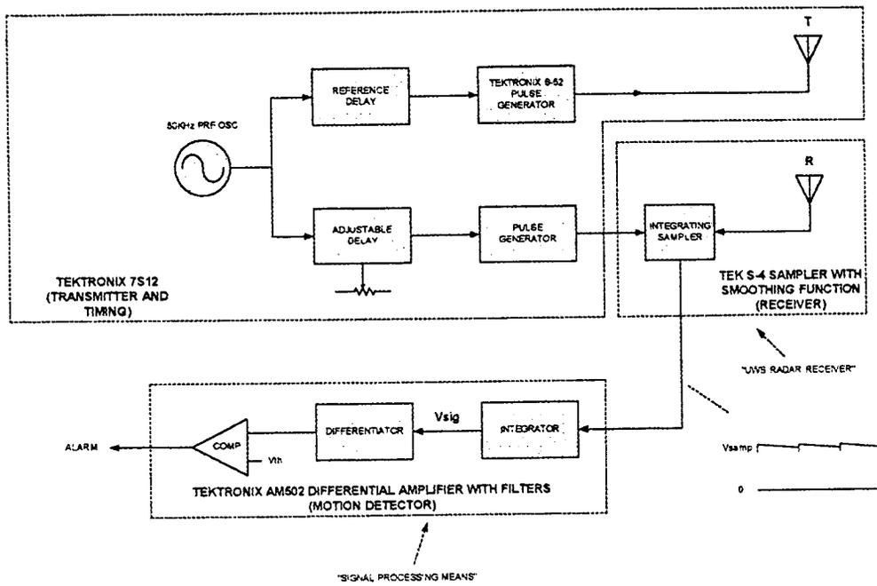
Fig. 4.0.5 UWB system constructed of purchased 1975 Tektronix components.
