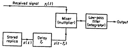
Figure 10.3 Block diagram of a cross-correlation receiver.
