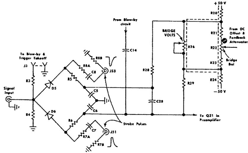
Fig. 4.0.3 Sampling Bridge Circuit and Bridge Volts and Bridge Bal Circuits. From *Tektronix Instruction Manual for Type S-2 Sampling Head*, Copyright 1968 by Tektronix, Inc., Beaverton, Oregon.
