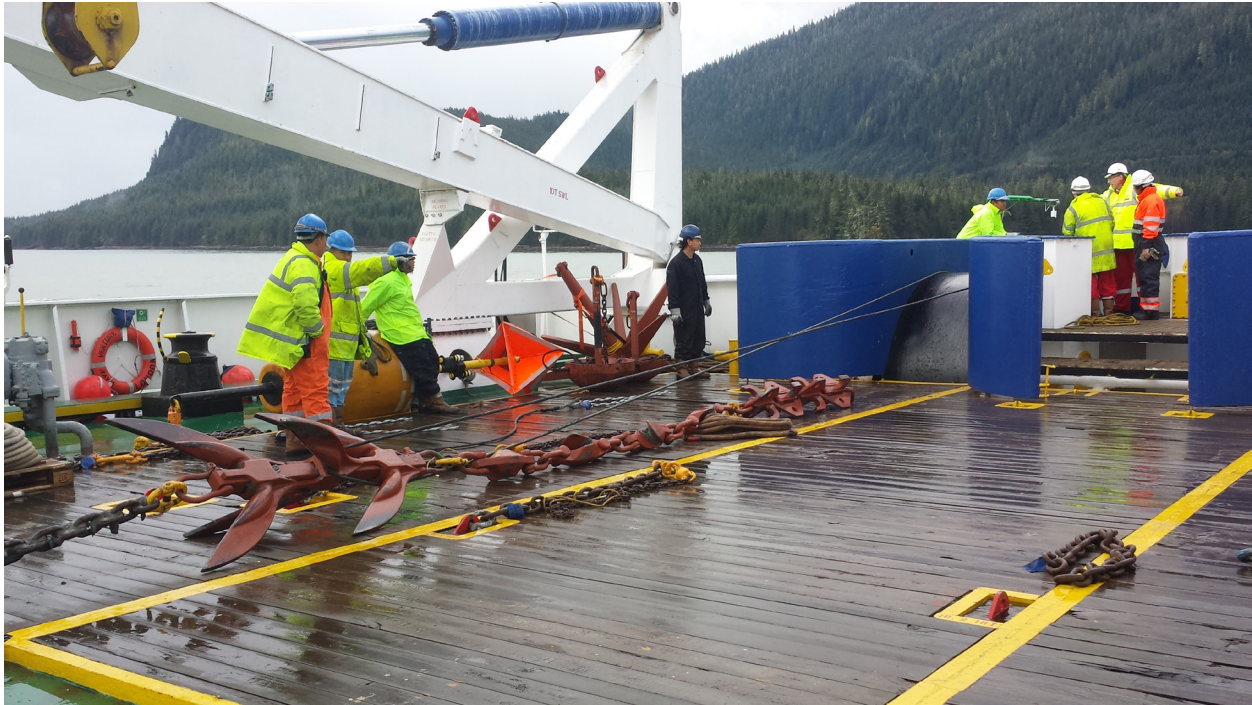
Figure 2-2. PLGR Grapnel on Board Cable Laying Ship
