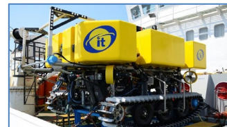
Photo 1. A ROVJET 207 remotely operated vehicle.
