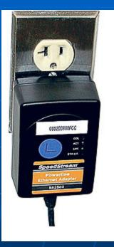
HomePlug Modem can turn an electrical outlet into an Internet connection.
