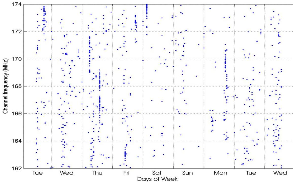
**Figure 2-2. Busiest Hour of the Week for Each Channel in the 162-174 MHz Band**
