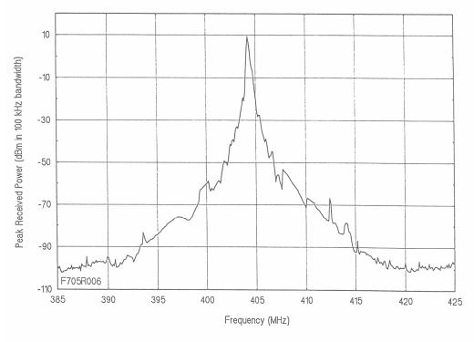
Figure 4-3. Platteville long-pulse radiated spectrum envelope.
