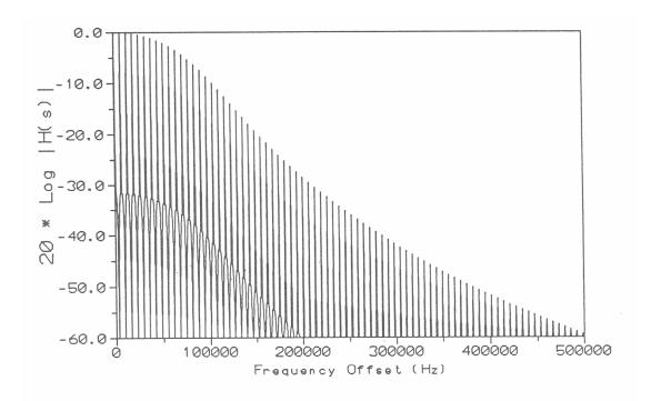
Figure 3-3. Oblique high mode frequency response.
