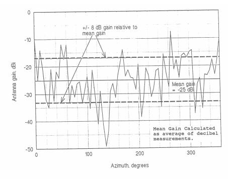
Figure 4-8. Platteville ground-level antenna pattern (east mode).
