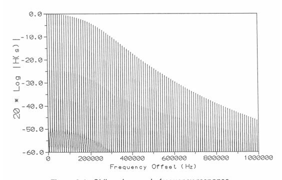
Figure 3-4. Oblique low mode frequency response.
