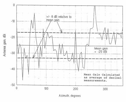
Figure 4-10. Platteville ground-level antenna pattern (vertical mode).
