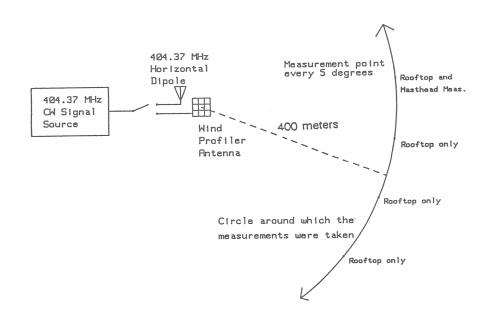
Figure 4-7. Antenna pattern measurement schematic.
