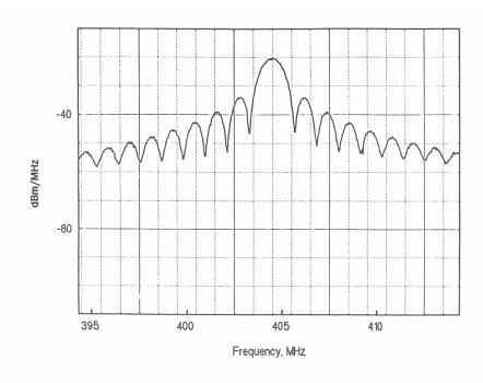
Figure 4-15. Non-FMed pulse spectrum, 1  $\mu$ s/pulse, 300 pps.
