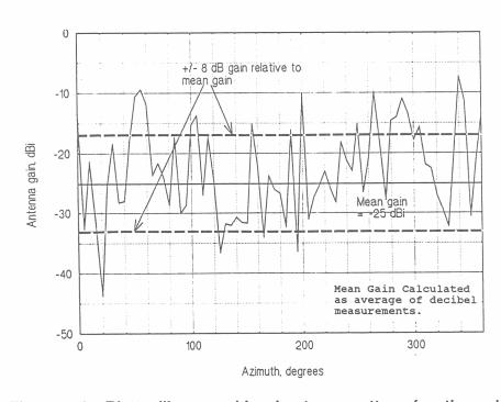
Figure 4-9. Platteville ground-level antenna pattern (north mode).
