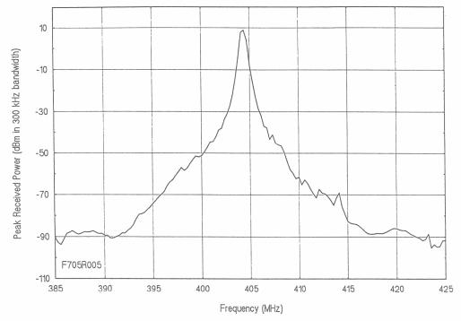
Figure 4-2. Platteville short-pulse radiated spectrum envelope.
