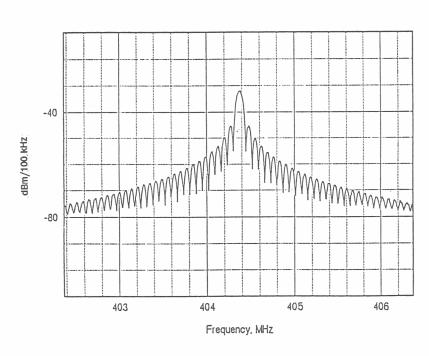
Figure 4-16. Non-FMed pulse spectrum, 10  $\mu$ s/pulse, 300 pps.
