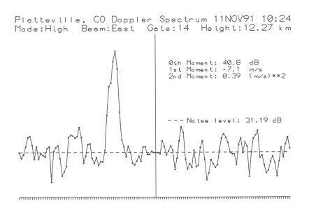
Figure 2-5. Profiler doppler spectrum.
