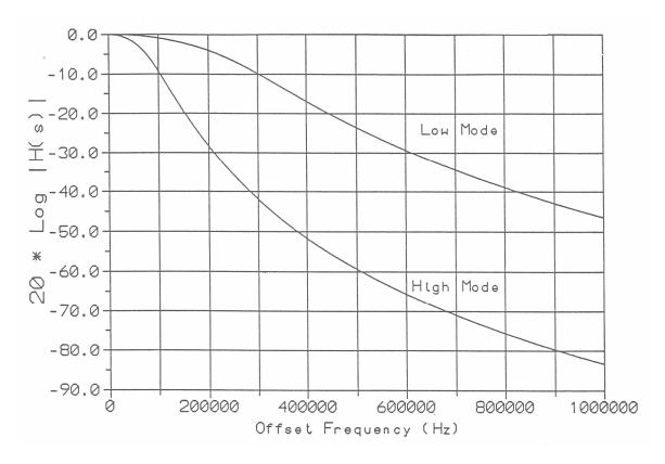
Figure 2-4. Frequency response of IF filters.
