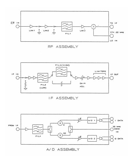
Figure 2-3. Profiler receiver block diagram.
