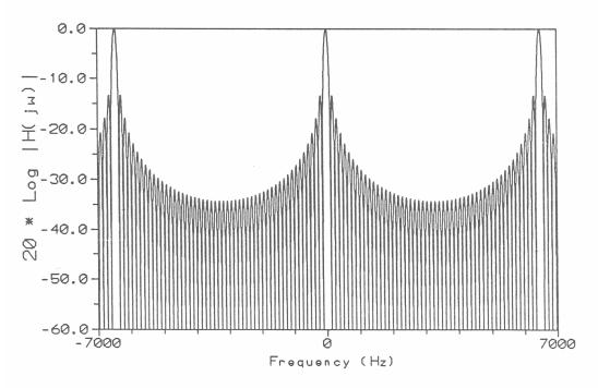
Figure 3-2. Oblique high mode frequency response ( $\pm$ 7000 Hz).
