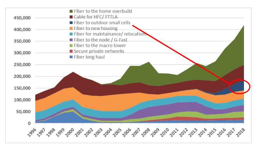
This is reviewing fiber route miles, i.e. the number of linear miles fiber is deployed overhead or underground – whether single or multiple fiber strands/ lines.
