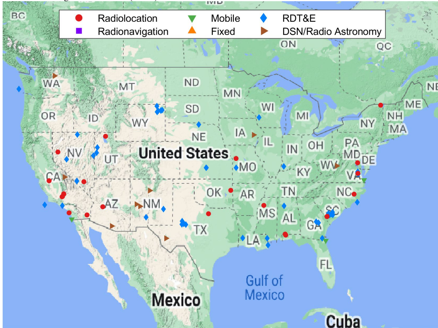
Figure 1: Federal Assignment Locations (Points) in 12.75-13.25 GHz
