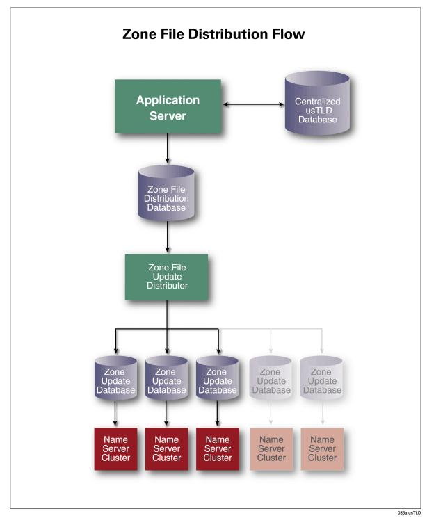
**Exhibit B.2-4.** NeuStar's process for near real-time updating of the nameserver zone file databases ensures that consistent and timely data are always available.
