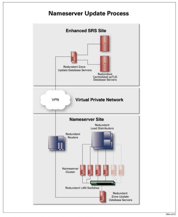
**Exhibit B.2-5.** Maintaining a zone file database at each nameserver data center allows zone file servers to respond to DNS inquiries by accessing their own local zone file database. This maximizes efficiency and increases redundancy.
