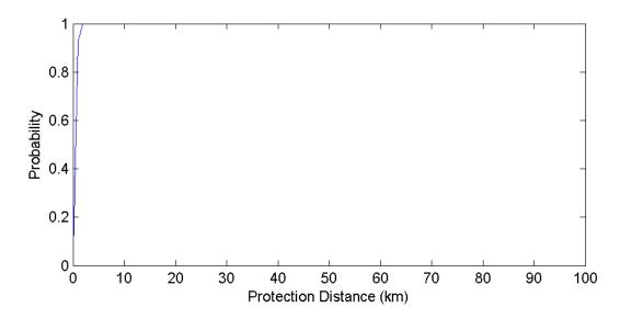
Figure 101. Boulder Colorado GOES Protection Distances – 10 MHz Channel (500 Iterations)
