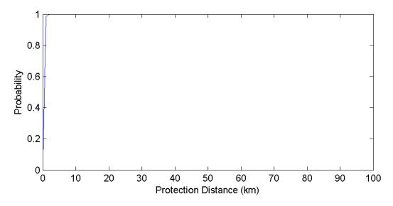
Figure 100. Boulder Colorado GOES Protection Distances – 5 MHz Channel (500 Iterations)
