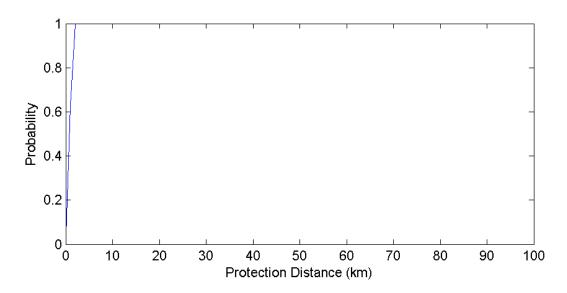
Figure 123. Norman Oklahoma GOES Protection Distances – 10 MHz Channel (500 Iterations)
