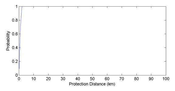
Figure 102. Boulder Colorado GOES Protection Distances – 15 MHz Channel (500 Iterations)
