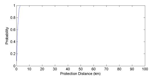
Figure 149. Offutt AFB Nebraska GOES-W Protection Distances – 5 MHz Channel (500 Iterations)
