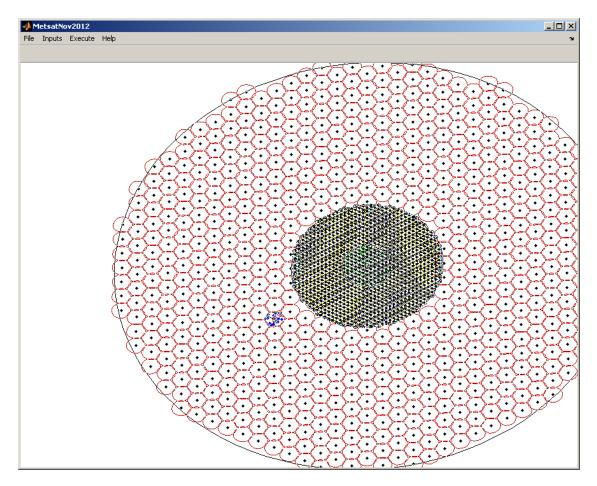
Figure 3. Example of Base Station Deployment Coverage Areas
