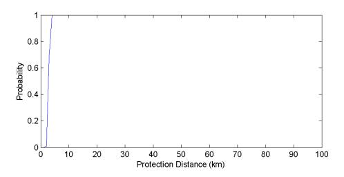
Figure 150. Offutt AFB Nebraska GOES-W Protection Distances – 10 MHz Channel (500 Iterations)
