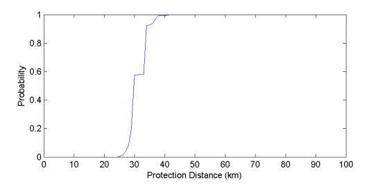
Figure 138. Guaynabo Puerto Rico GOES Protection Distances – 10 MHz Channel (500 Iterations)
