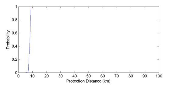
Figure 156. Anderson AFB Guam POES Protection Distances – 10 MHz Channel (500 Iterations)
