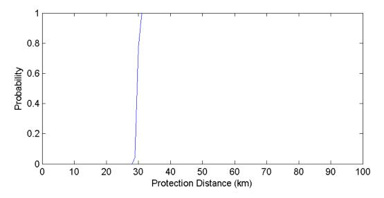
Figure 91. Barrow Alaska POES Protection Distances – 5 MHz Channel (500 Iterations)
