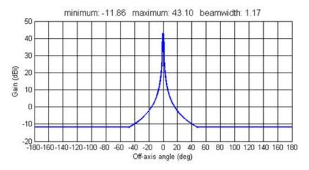
Figure 1. Azimuth and Elevation Antenna Pattern
