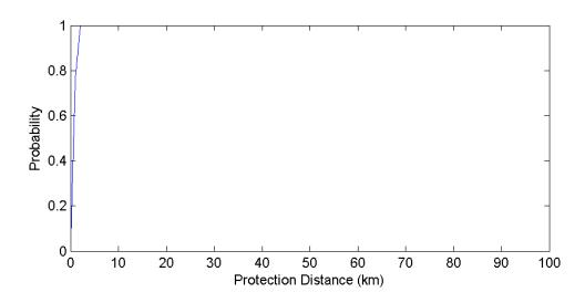
Figure 132. Sioux Falls South Dakota GOES Protection Distances – 10 MHz Channel (500 Iterations)
